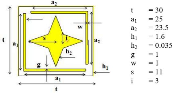
Fig. 2. Illustration of unit cell of proposed RFID crack sensor [9]. All dimensions are in mm.
