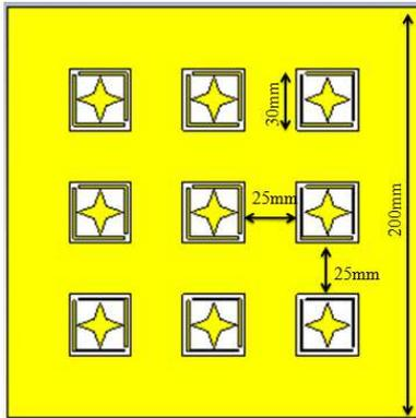
Fig. 3. Geometry of  $3 \times 3$  array configuration.
