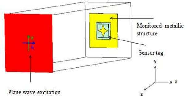
Fig. 5. Simulation setup for RCS measurement in CST Microwave Studio [9].
