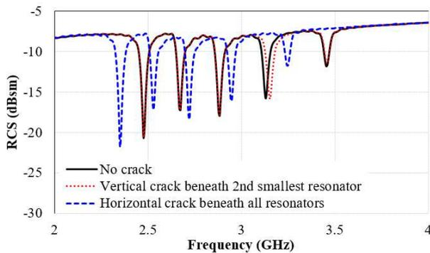
Fig. 8. Simulated RCS responses of series array of non-identical rectangular resonators.
