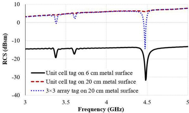
Fig. 7. Comparison of RCS responses of unit cell and 3×3 array of proposed sensor tags.
