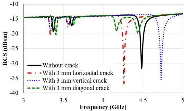
Fig. 6. Simulated RCS responses of unit cell sensor tag.
