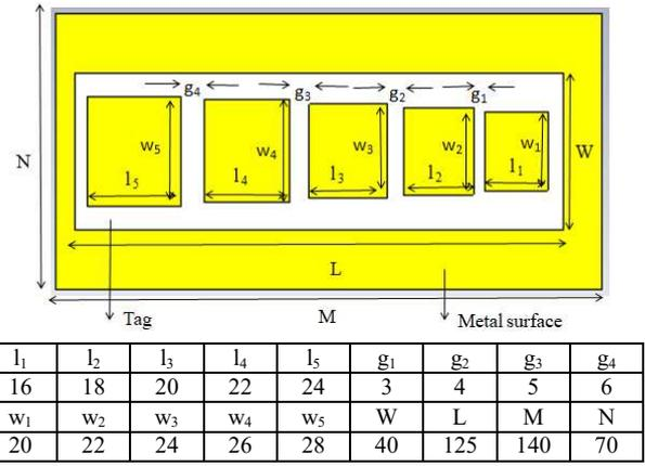
Fig. 4. Geometry of series array RFID sensor tag for metal crack detection. All dimensions are in mm.
