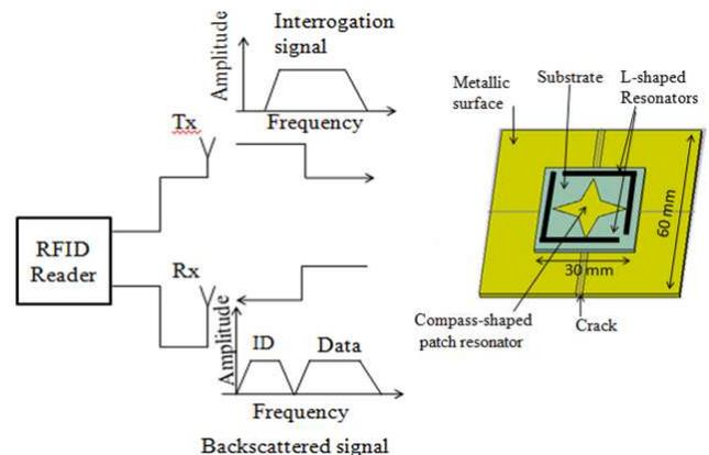
Fig. 1. Schematic of working principle of RFID system [9].
