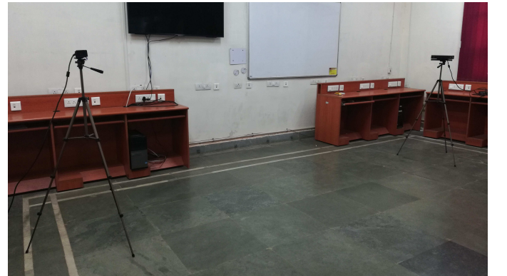
Fig. 4: Camera setup for data collection using two Kinect cameras for the front and back views
