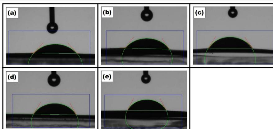
Fig.5 Water contact angle of the TKP/PSO films
