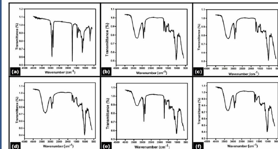
Fig.6 FTIR profile of TKP/PSO
