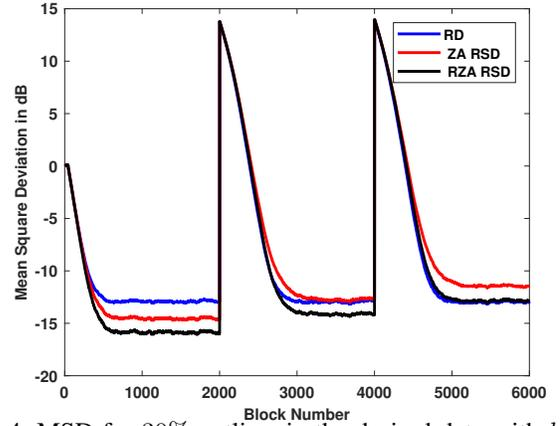
Fig. 4: MSD for 30% outliers in the desired data with  $k = 50$
