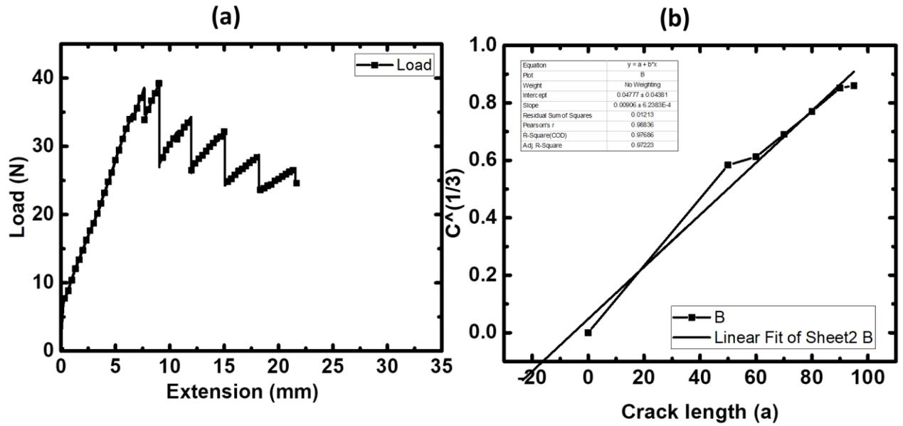
Figure 8. (a) Load vs. displacement curve and (b) Compliance vs. crack length curve
