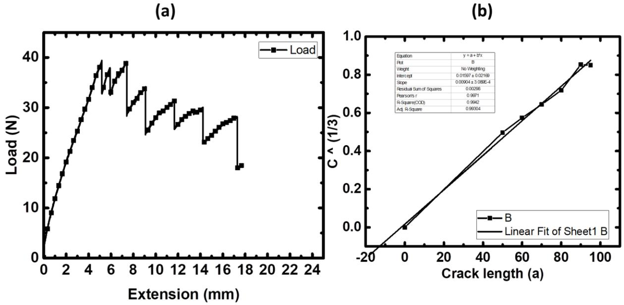
Figure 6. (a) Load vs. displacement curve and (b) Compliance vs. crack length curve
