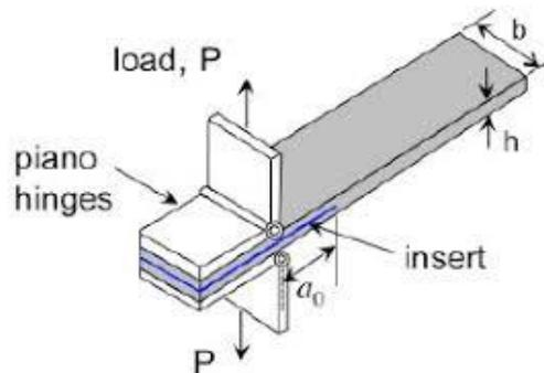
Figure 2. DCB test set-up for Mode-I ILFT
