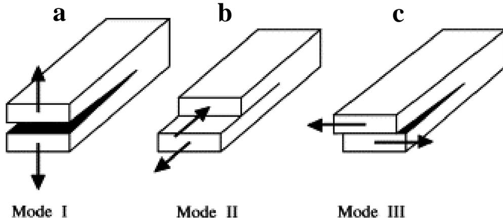
Figure 1. (a) Tensile load, (b) Shear load, and (c) torsion load
