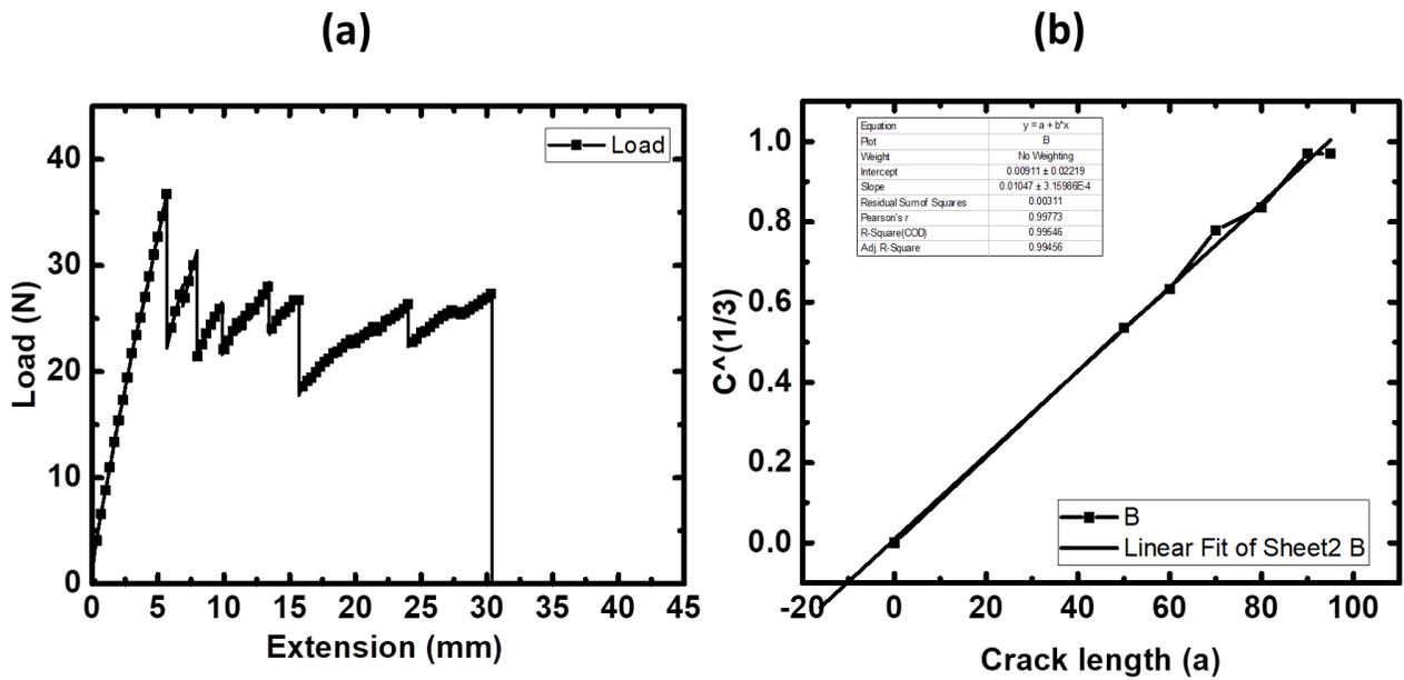
Figure 7. (a) Load vs. displacement curve and (b) Compliance vs. crack length curve
