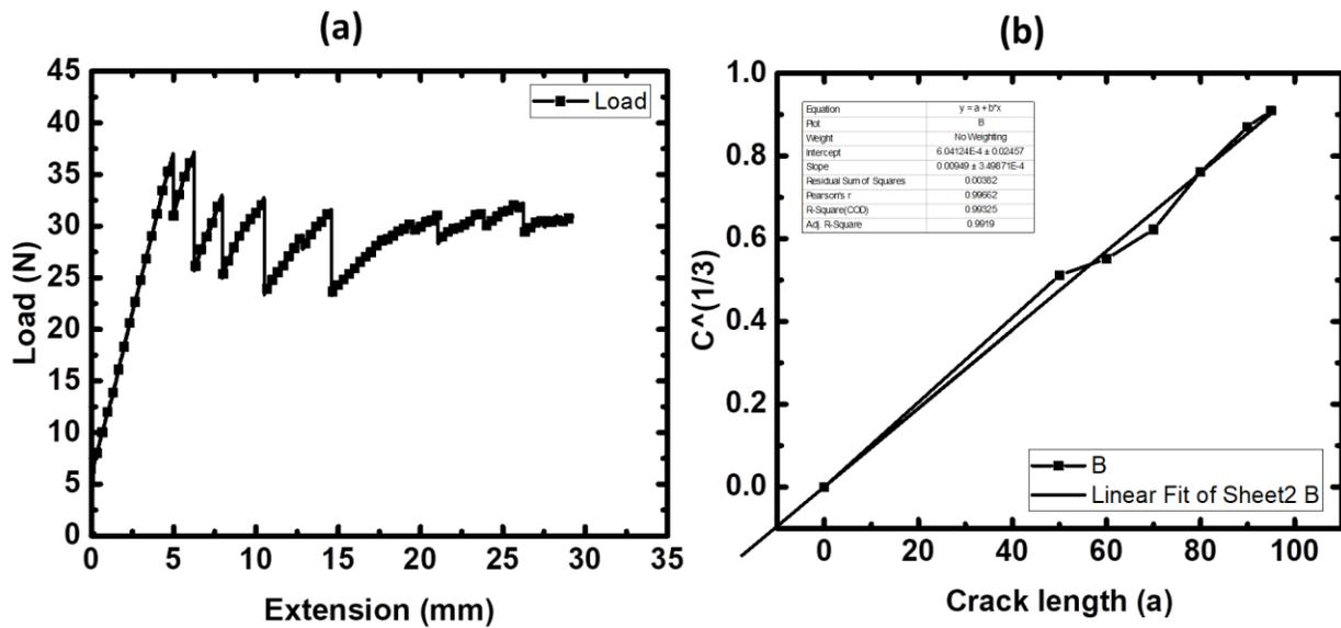
Figure 5. (a) Load vs. displacement curve and (b) Compliance vs. crack length curve
