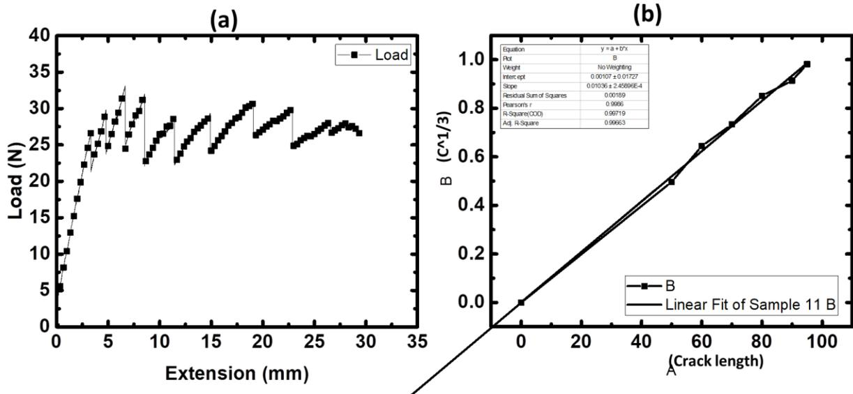
Figure 4. (a) Load vs. displacement curve and (b) Compliance vs. crack length curve
