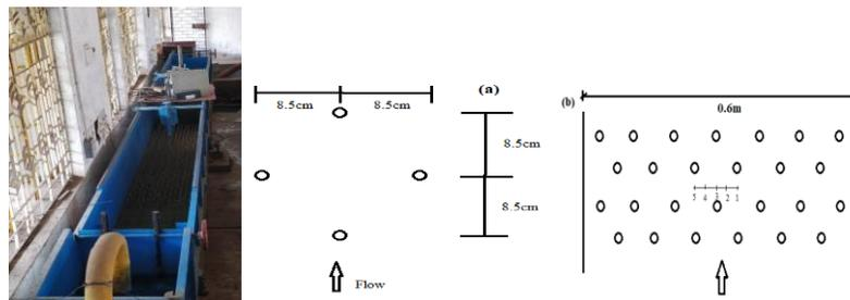
**Figure 2.** Photographs of the experimental set-up and staggered rigid vegetation pattern, H. E. Lab., NITR
