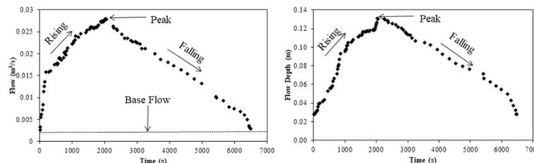
**Figure 4.** Flow and depth hydrograph in an unsteady flow run
