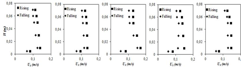
Figure 6. Velocity profiles for lower flow depth case (left to right: location 1 to location 5)
