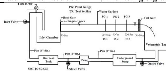
**Figure 1.** A schematic diagram of the experimental setup, NITR
