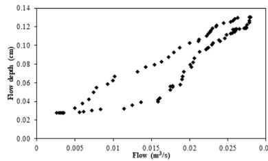
Figure 5. Hysteresis plot of stage-discharge curve
