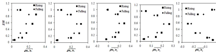
Figure 7. Distribution of vertical Reynolds stress for lower flow depth case (left to right: location 1 to location 5)
