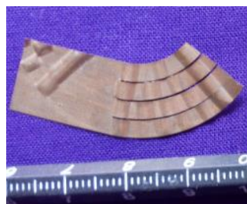
Figure 5: Fabricated thrust bump foils
