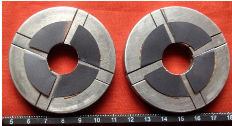
Figure 7: Assembled lower and upper gas foil thrust bearing with layer of MoS 2 coating on top foil. The fabricated bump foil is fixed with the grub screw as shown in Fig 6. The top foil with a coating of MoS 2 is mechanically fitted with the bearing base as shown in Fig 7.
