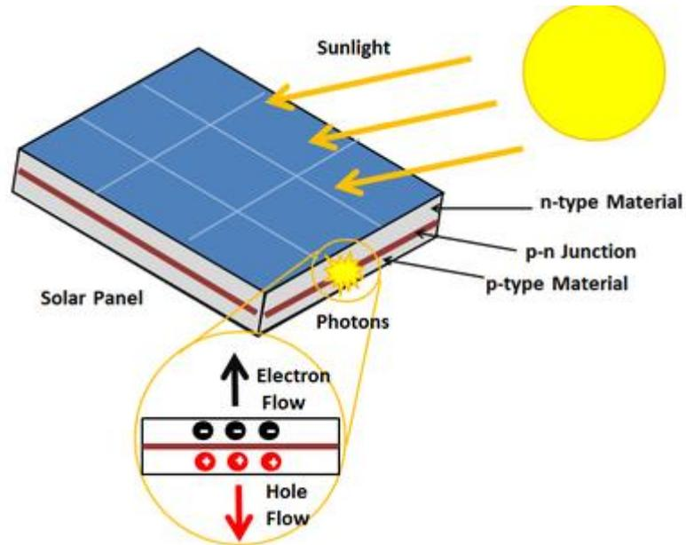
Photovoltaics is the conversion of light into electricity using semiconducting materials
