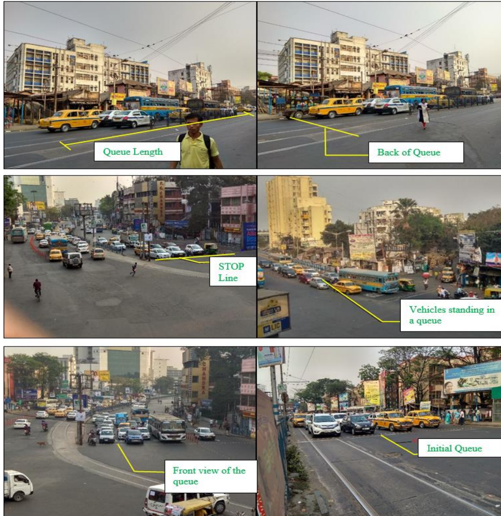
FIGURE 1 Different parameters considered for Queue length estimation
