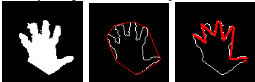
Figure 9 Input Binary Image, Convex Hull (red) and Convexity Defects illustrated in image
