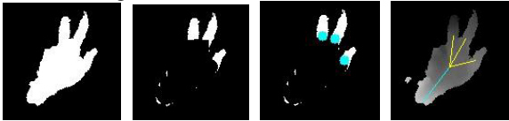
Figure 8 Input binary image, Top Hat Transform, Feature Points and Features as angle between yellow and blue lines
