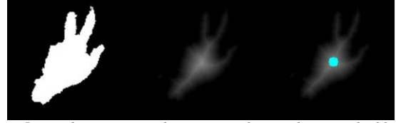
Figure 5 Input binary image, distance transform and maxima highlighted as center of palm
