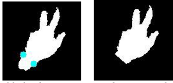
Figure 7 Highlighted Wrist Points and gesture without hand part
