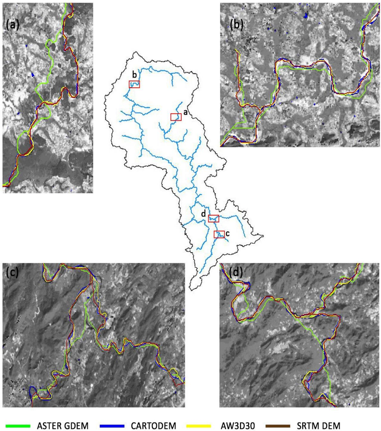
**Figure 2.** River network delineation by different DEM sources.
