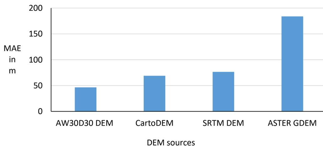
**Figure 3.** MAE error due to DEM sources in Jeraikelela catchment
