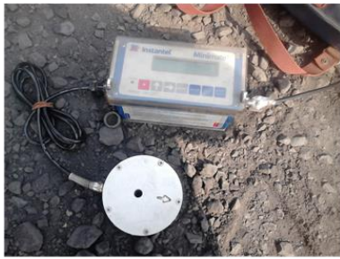
Figure 6: Minimate Blaster, an Instrumentation installed at a typical blast site
