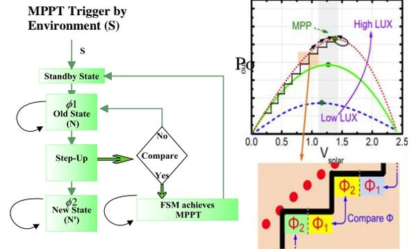
Fig. 5. Flow chart of Hill-Climbing Algorithm with procedure
