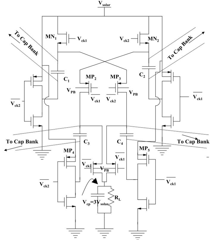
Fig. 4. Circuit diagram of Charge Pump as a Voltage Tripler
