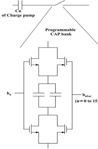
Fig. 6. Digitally programmable capacitor bank
