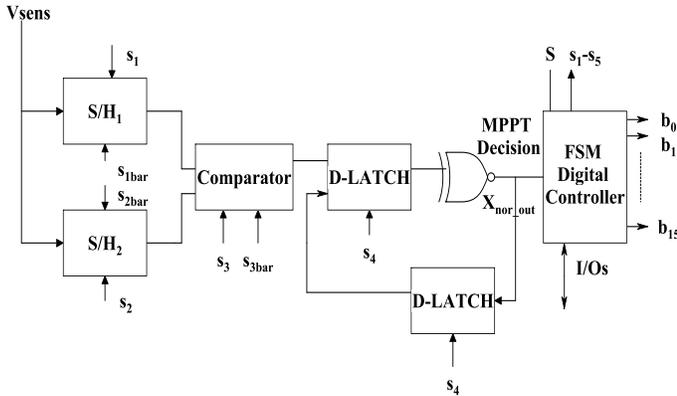
Fig. 7. MPPT procedure with FSM
