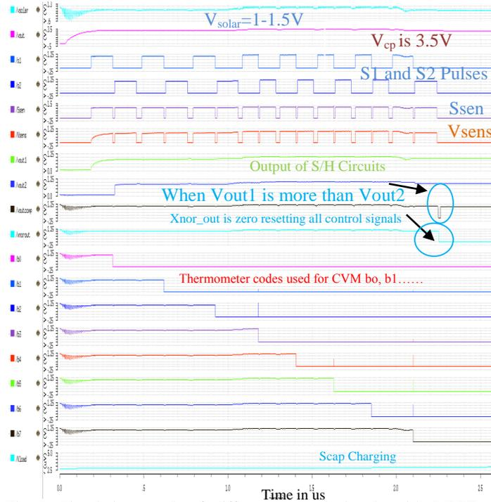
Fig 9. Simulation result of different control signals with MPPT achievement
