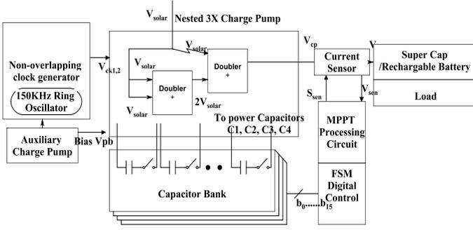
Fig. 1. Block Diagram of Energy Harvesting System
