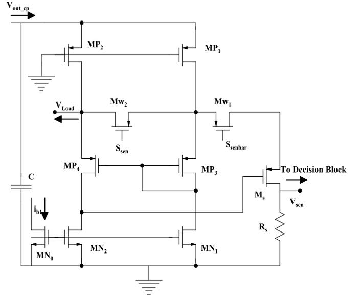
Fig. 8. Energy efficient Current Sensor
