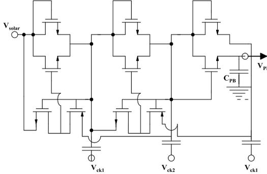
Fig. 2. Circuit Diagram of Auxiliary Charge Pump for Bias generation
