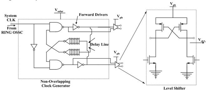
Fig. 3. Circuit diagram of Non-overlapping Clock generator with Level Shifter
