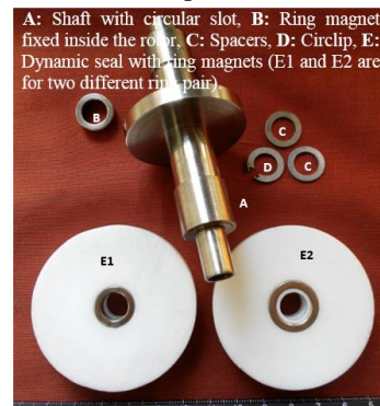
Fig. 2. Fabricated rotor and passive axial magnetic bearing for turboexpander.
