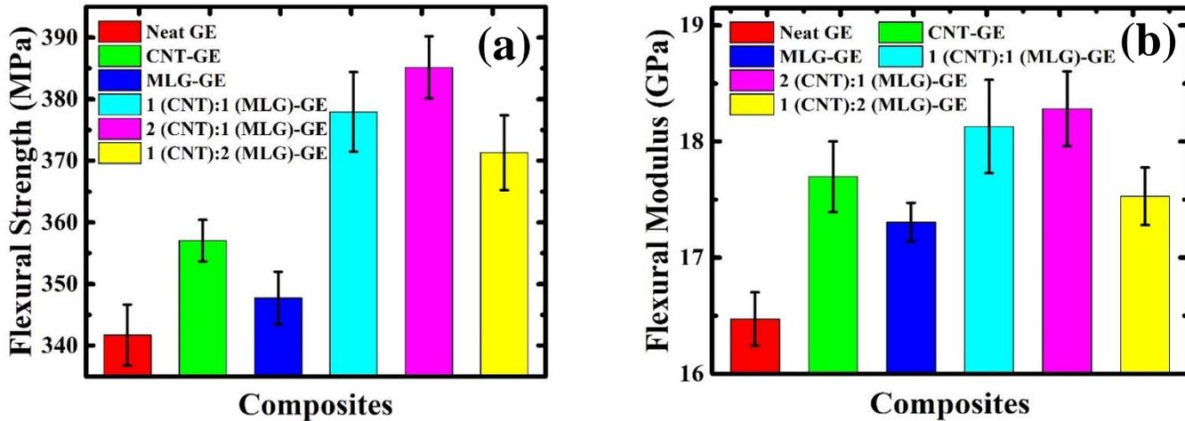
Fig.1. Diversification of a) flexural strength b) flexural modulus with different CNT-MLG contents embedded in GE composite
