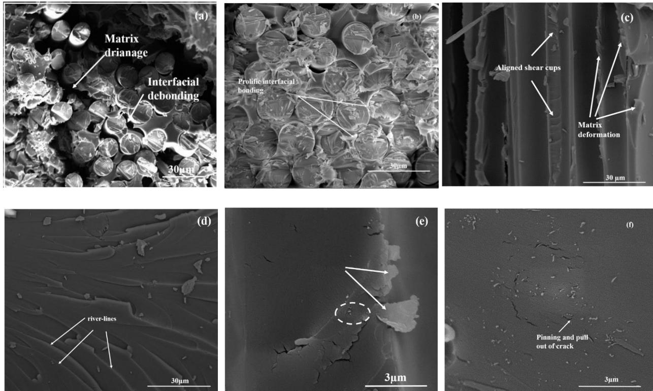
Fig.3. Depicts the FESEM images of deformation behaviour, interfacial zone, crack mechanism of a) GE composite embedded with b, d) CNT:MLG(2:1), C, f)CNT:MLG(1:1), d, e)CNT:MLG(1:2) nanofillers.
