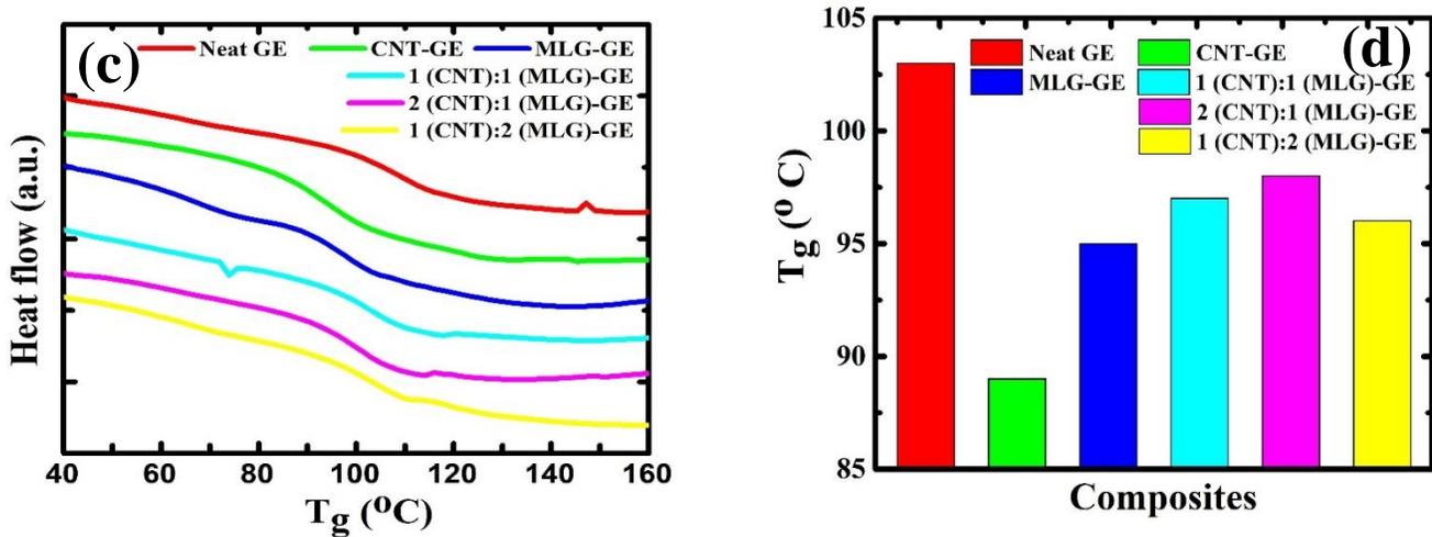
Fig.2. Depicts the c) DSC analysis, d) diversification of glass transition temperature by incorporating different ratios of CNT-MLG in GE composite
