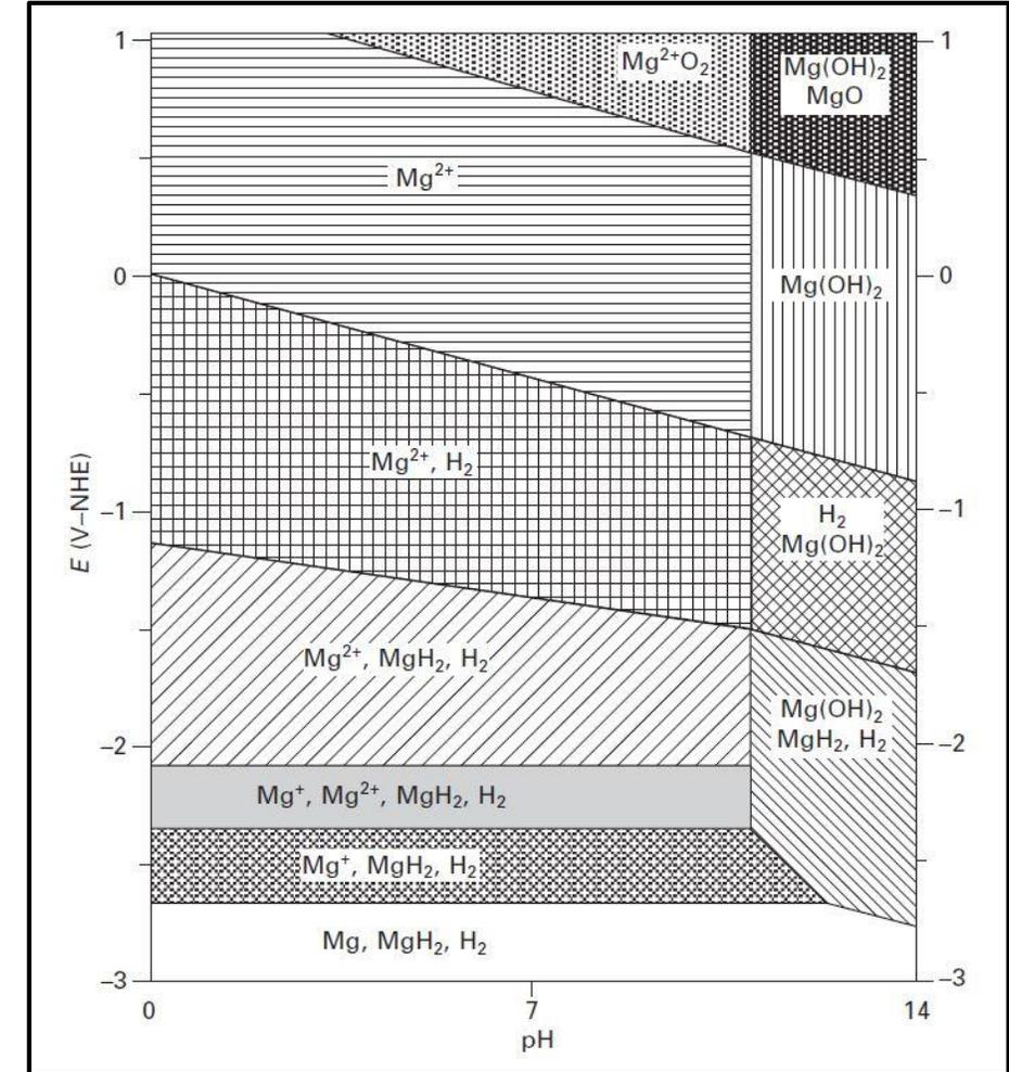
E-pH diagram with possible stable substances in a Mg-H<sub>2</sub>O electrochemical system.
