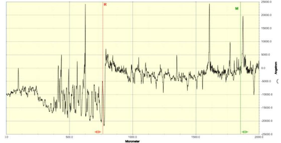
Image showing the graphical representation for CeCC for 30s on Mg-4Y sample using stylus surface profilometer
