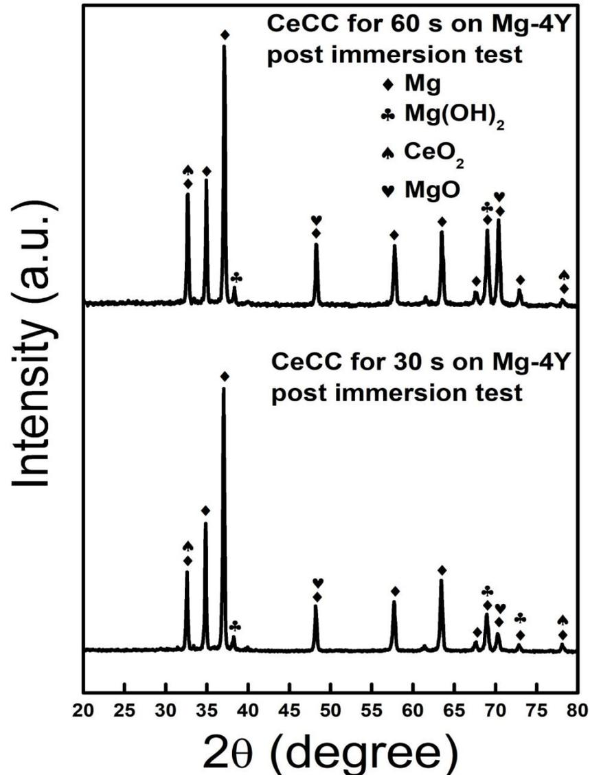
The XRD patterns showed high intensity base metal peaks along with the low intensity peaks of CeO<sub>2</sub> confirming the presence of CeO<sub>2</sub> deposition on the base metal surface with the formation of oxides (MgO and Mg(OH)<sub>2</sub>) on Mg after corrosion.
