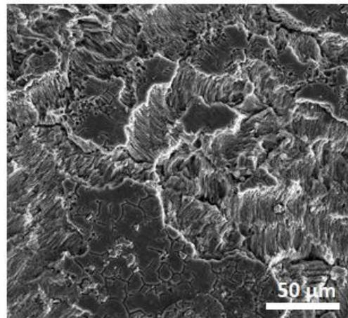
For the Mg-4Y\_30s samples, crevices appeared but as the CeCC duration increased the crevices aggressively started penetrating in the alloy underneath and started forming deep corrosion pits.
