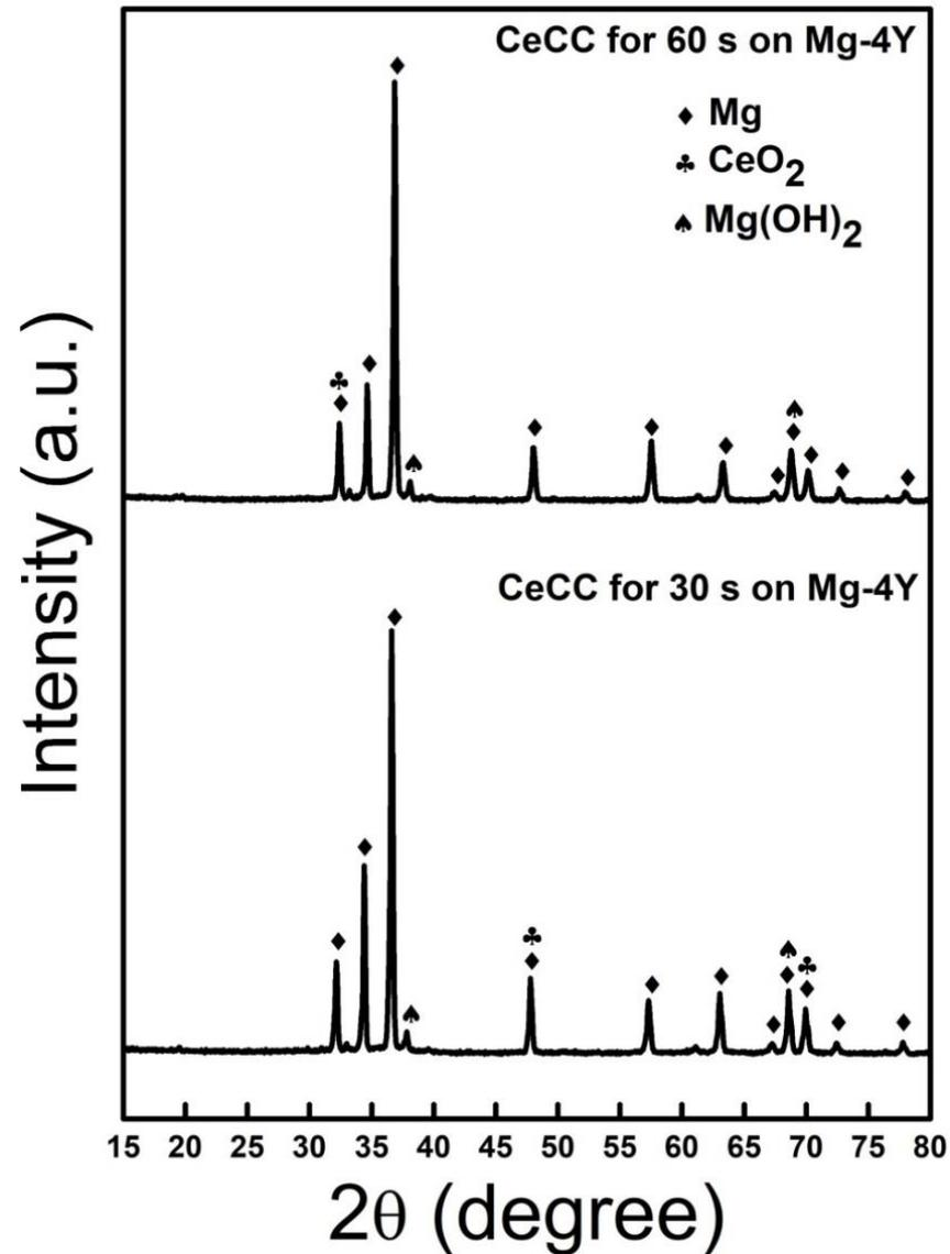
The base metal peaks appeared at high intensity along with the low intensity peaks of CeO<sub>2</sub> and Mg(OH)<sub>2</sub> confirming the presence of CeO<sub>2</sub> deposition on the base metal.
