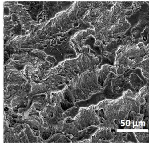
For the bare Mg-4Y sample, corrosion pits were formed with adjoining boundaries on the surface.
