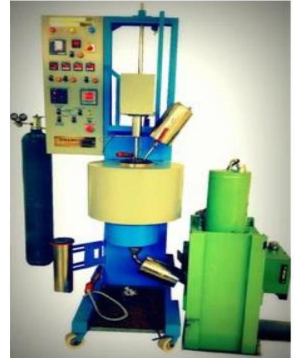
Fig. Bottom pouring type stir casting furnace with squeeze casting setup
