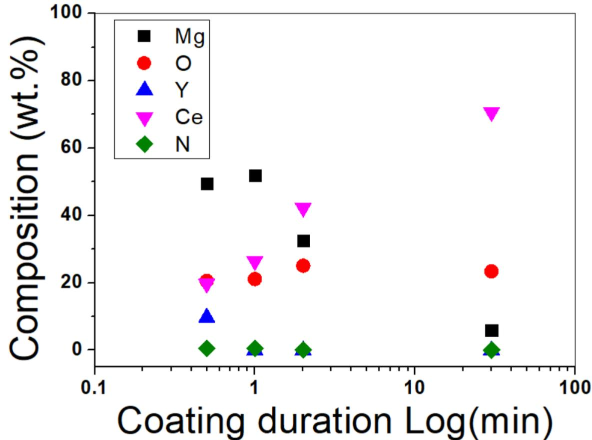
The amount of nitrogen was negligible with marginal lowering of Yttrium content throughout the coating duration. In addition, the amounts of Oxygen and Cerium were increasing with the increasing coating duration.
