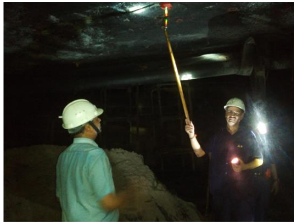
Fig 6: Dual height tell tail instrument in the Stowing panel for observation of tendency of bed separation in the parting between 3 and 4 seams at GDK 11 mine
