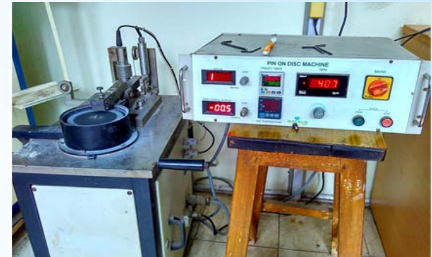
Figure 3: Experimental set up of pin-on-disc wear tester.
