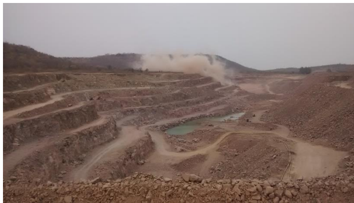
Fig 1: A view of blasting in trial blast and working benches at Dunguri mine, ACC
