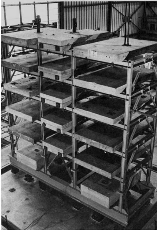
Fig. 2 Experimental model of five-storey steel frame adopted from literature [13].
