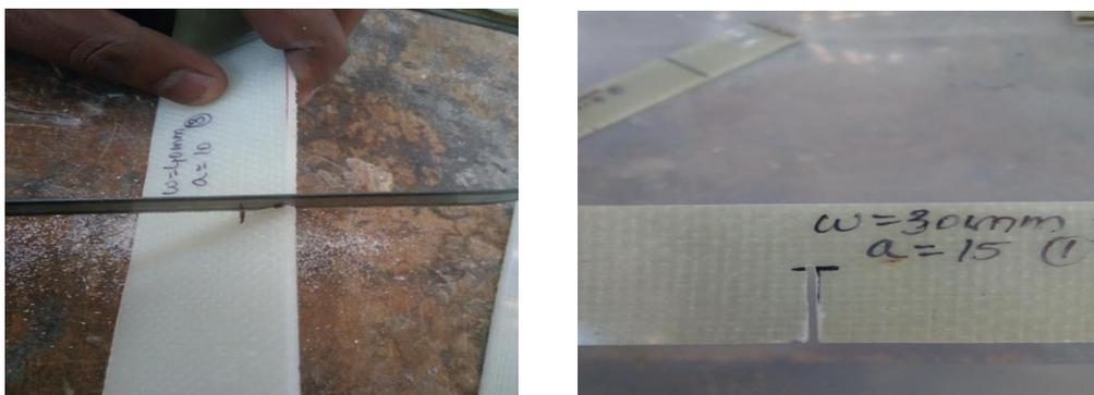
Fig. 2. (a) Introducing a crack with hacksaw blade; (b) Specimen after introducing a crack
