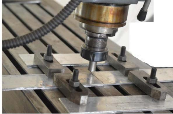
Fig.1. Experimental arrangement on vertical milling machine
