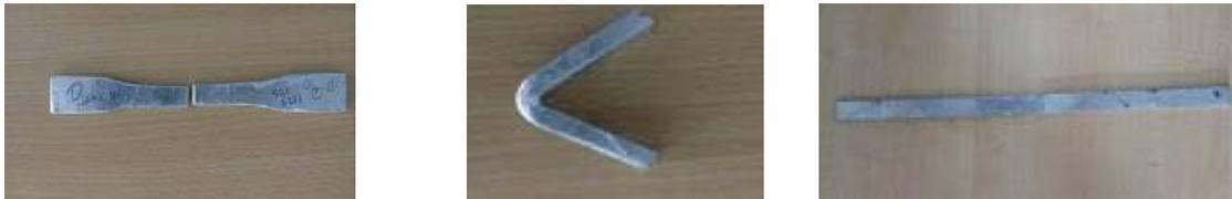
Fig.2. Test samples in one condition (22 mm/min, 760 rpm, 2.2 mm depth)
