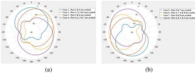
Fig. 10: Measured radiation patterns of PPMFMA at 1.03 GHz - (a) case 1 to case 4 and, (b) case 5 to case 8.
