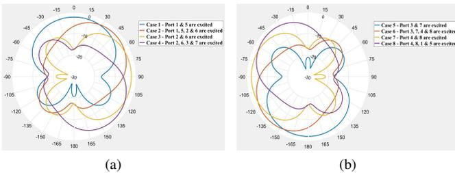
Fig. 11: Simulated radiation patterns of PPMFMA at 1.09 GHz - (a) case 1 to case 4 and, (b) case 5 to case 8.
