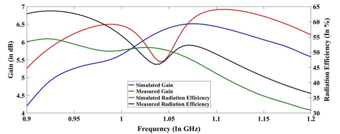
Fig. 7: Gain and radiation efficiency plot of PPMFMA.
