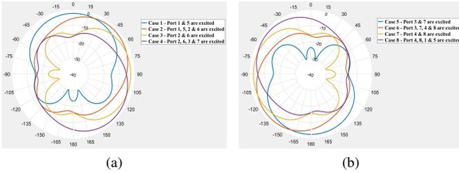
Fig. 9: Simulated radiation patterns of PPMFMA at 1.03 GHz - (a) case 1 to case 4 and, (b) case 5 to case 8.
