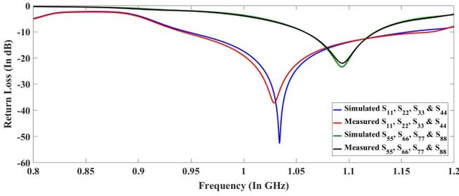
Fig. 8: Simulated and measured return loss of PPMFMA.
