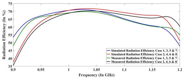
Fig. 14: Radiation efficiency vs frequency plot of PPMFMA.
