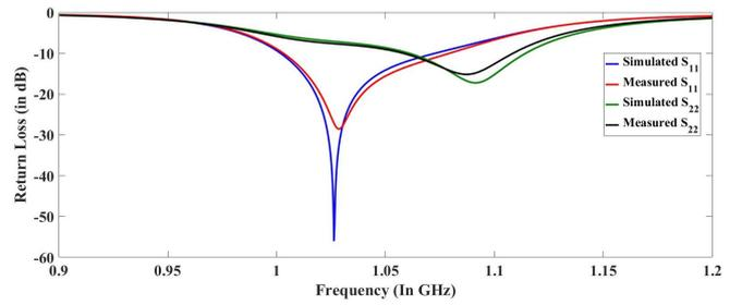
Fig. 5: Simulated and measured return loss of DPDFMA.
