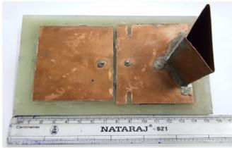
Fig. 2: Fabricated model of DPDFMA.
