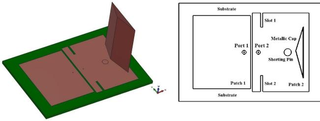
Fig. 1: Simulated and schematic model of DPDFMA.
