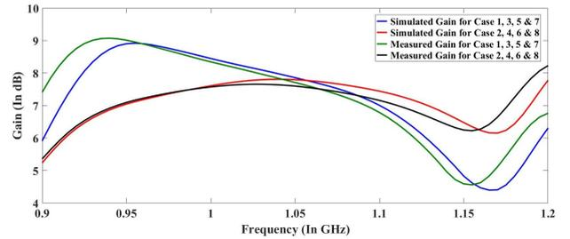
Fig. 13: Gain vs frequency plot of PPMFMA.
