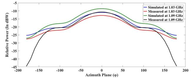
Fig. 6: Simulated and measured power patterns of DPDFMA.
