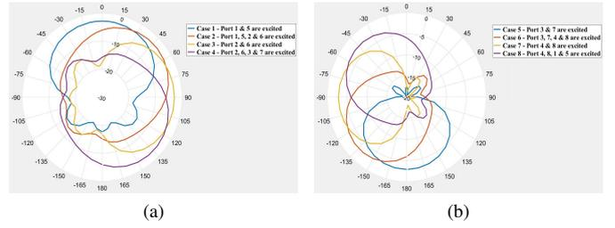
Fig. 12: Measured radiation patterns of PPMFMA at 1.09 GHz - (a) case 1 to case 4 and, (b) case 5 to case 8.
