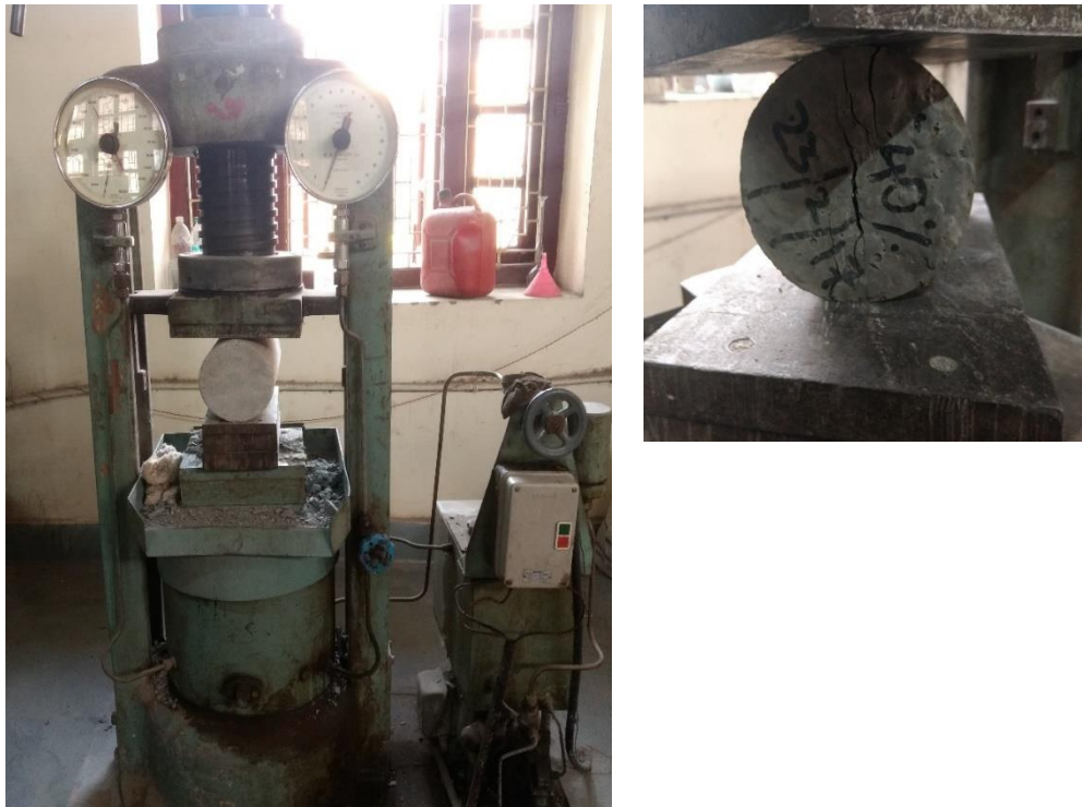
Figure 2: Experimental Setup for Split Tensile Strength of concrete cylinder
