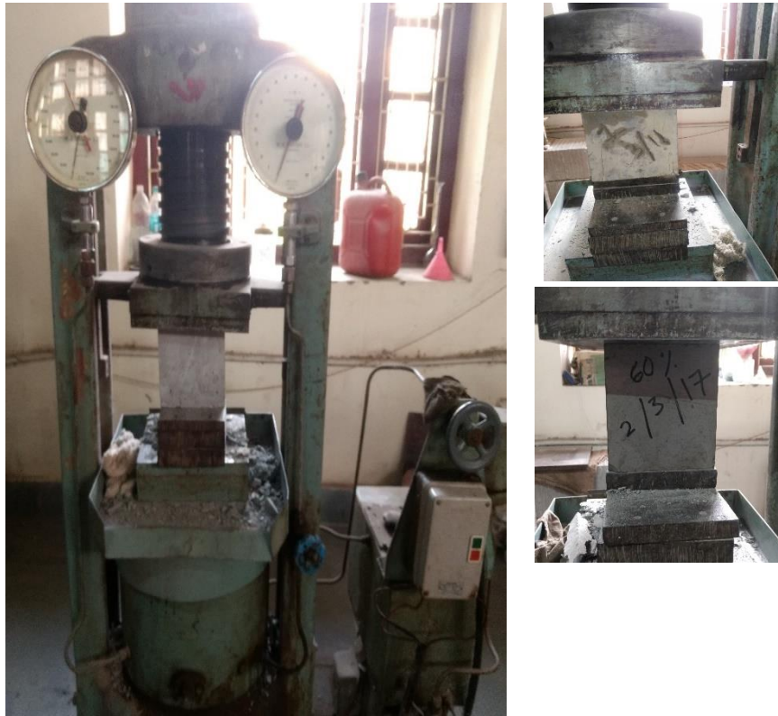
Figure 1: Experimental Setup for Compressive Strength of concrete
