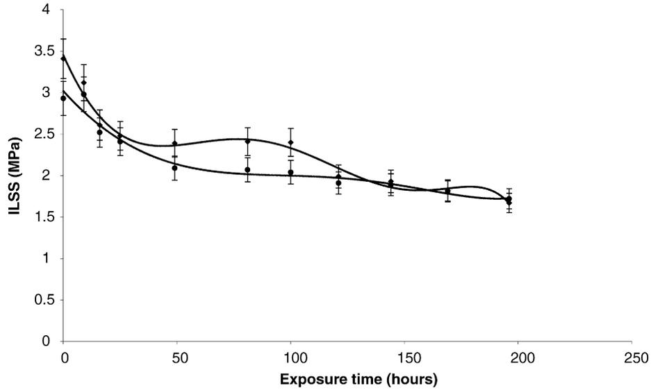
Fig. 3. Variation of ILSS values with exposure time of frozen hygrothermally conditioned glass fibre/epoxy composite for different loading speeds ((●) 1 mm/min and (◆) 10 mm/min).
