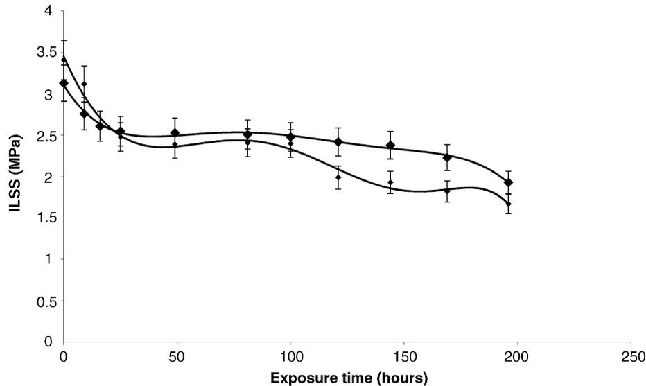
Fig. 5. Comparison of ILSS values of plain moisture and frozen moisture conditioned glass fibre/epoxy composite at 10 mm/min crosshead speed ((◆) frozen moisture and (●) plain moisture).
