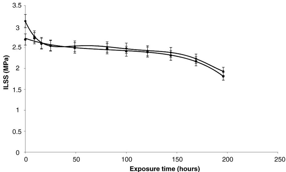
Fig. 2. Variation of ILSS values with exposure time of glass fibre/epoxy composite for different loading speeds (●) 1 mm/min and (◆) 10 mm/min.
