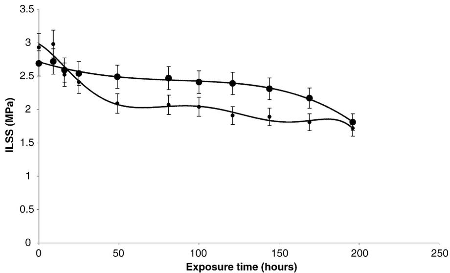
Fig. 4. Comparison of ILSS values of plain moisture and frozen moisture conditioned glass fibre/epoxy composite at 1 mm/min crosshead speed ((●) frozen moisture and (●) plain moisture).
