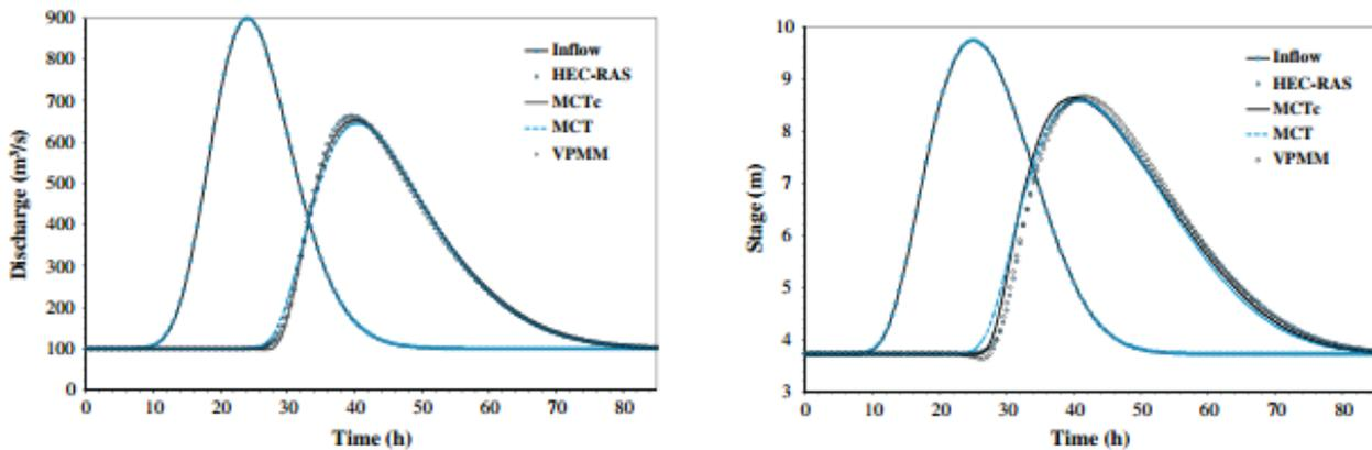
2)  $\Delta x=2$ , Reproduction of the benchmark discharge hydrograph by the VPMM, MCT and  $MCT_c$  methods corresponding to 50 sub reaches. (M. Perumal, 2013)
