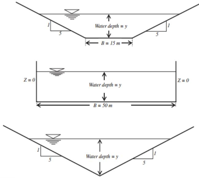
Fig. - prismatic cross-sectional shapes of routing reaches in the numerical experiments. (M. Perumal, 2013)
