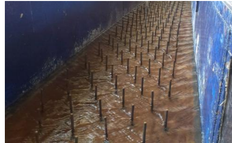
Figure 3: Arrangement of rigid rods as vegetation in experimental flume
