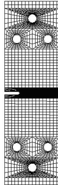
Fig.3a. Resulting mesh of the present simulation
