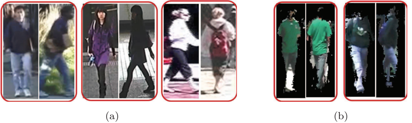
Figure 13: (a) Image-pairs with drastic pose and viewpoint variations, (b) Image-pairs with improper background removal
