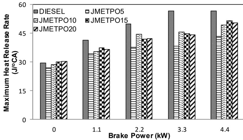
Fig. 6 Variation of maximum heat release rate with brake power
