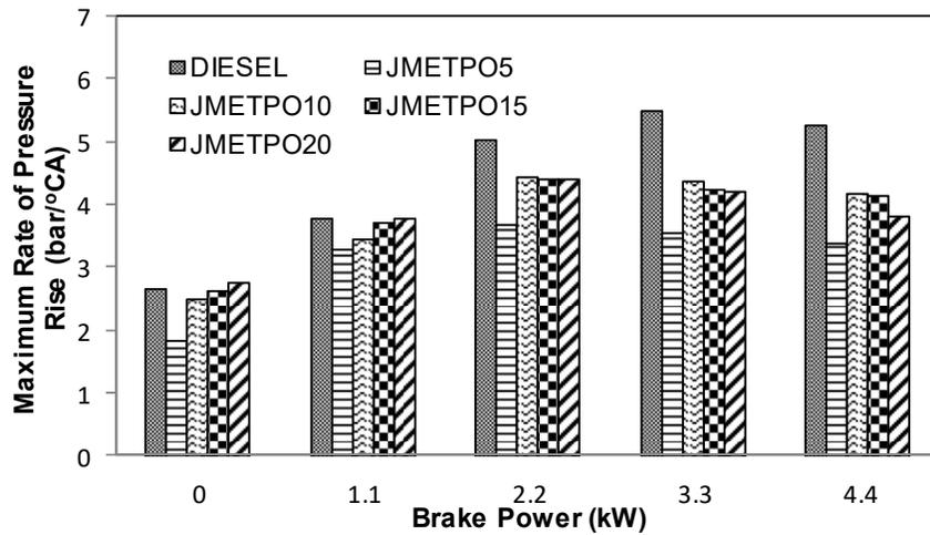
Fig. 9 Variation of maximum rate of pressure rise with brake power
