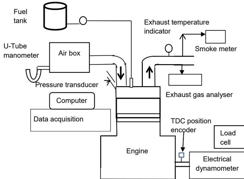
Fig. 2 Experimental setup
