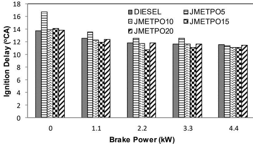
Fig. 4 Variation of ignition delay with brake power
