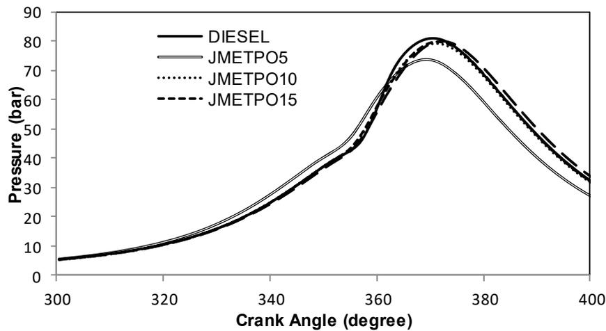
Fig. 3 Variation of cylinder pressure with crank angle
