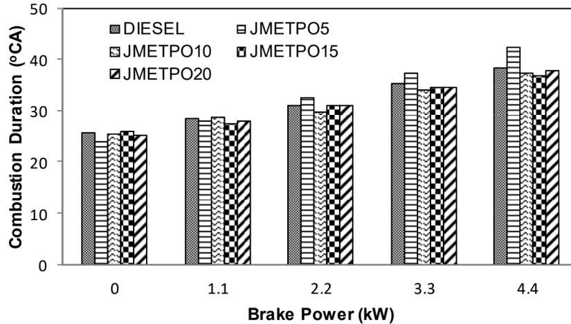
Fig. 7 Variation of combustion duration with brake power
