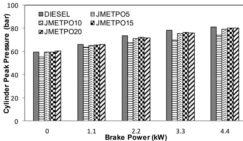
Fig. 8 Variation of cylinder peak pressure with brake power
