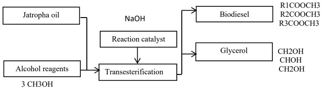
Fig. 1 Schematic diagram of the transesterification process
