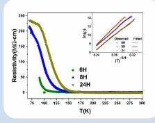
\* The temperature dependent resistivity in the temperature range of 70K to 300K. Inset shows linear fit (solid lines) of  $\ln \rho$  vs T<sup>-1/4</sup> plot
