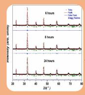
Rietveld refined x - ray diffraction data for La<sub>2</sub>NiMnO<sub>6</sub> samples sintered at various temperature are shown in the right figure.
