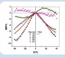
\* The field dependent magnetoresistance at 150, 200, 275 and 300K of the 24 hours sintered LNMO.
