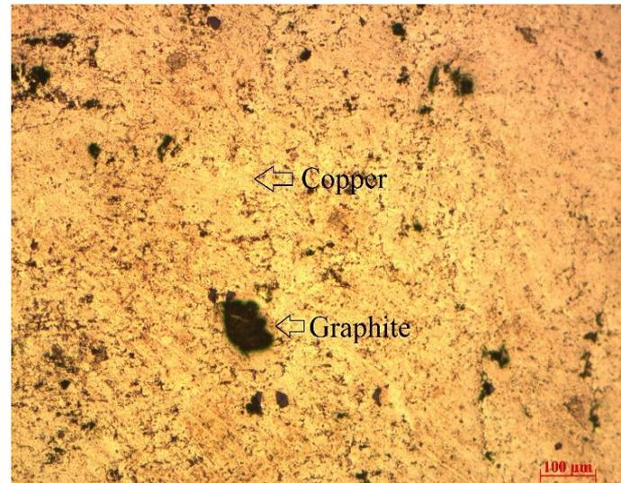
*Optical micrograph of Cu-5 vol.% Graphite*
