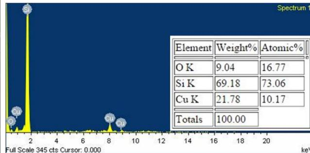
SEM-EDX analysis of wear debris of (a) Cu-5 vol. % gr-5 wt. % SiC, (b) Cu-5 wt. % SiC
