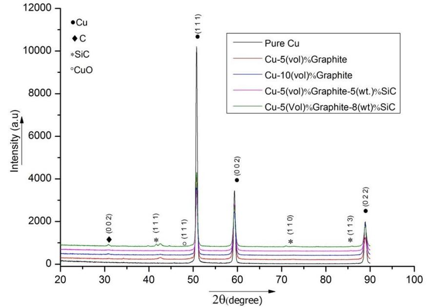
XRD spectra of rolled composites
