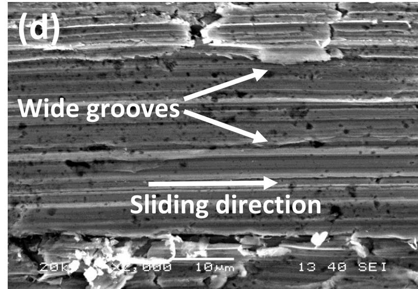
SEM micrographs of wear track of Cu-5 vol. % gr-5 wt. % SiC when (a and c) 20N and (b and d) 40N load applied
