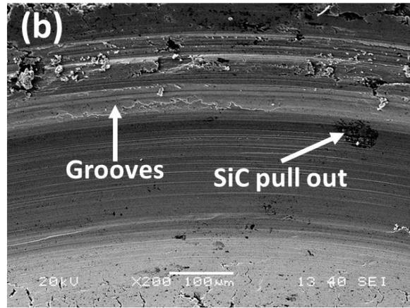
SEM micrograph of worn surface (a) Pure Cu, (b) Cu-5 wt. % SiC
