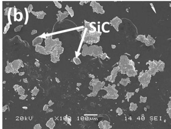
Wear debris of (a) Pure Cu, (b) Cu-3 vol. % graphite-5 wt. % SiC
