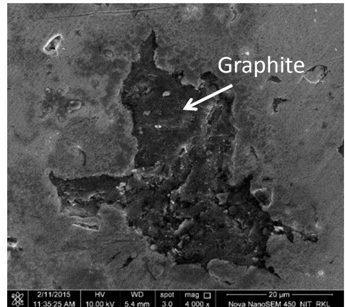
FESEM micrograph of Cu-5vol. % graphite-5wt.% SiC composite
