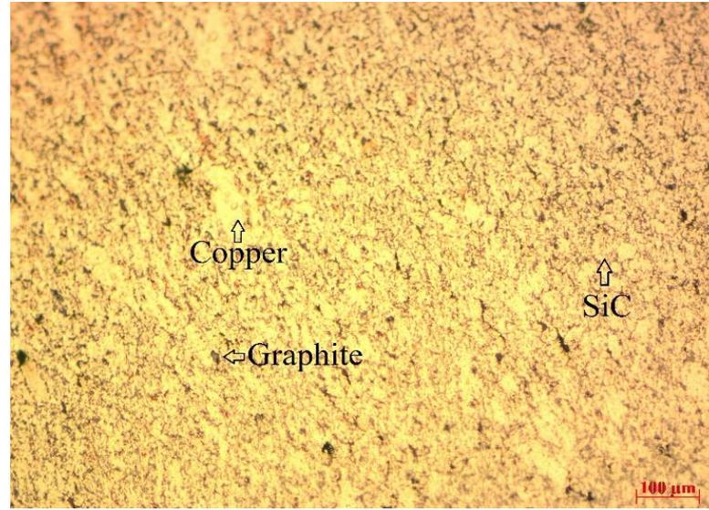
*Optical micrograph of Cu-5 vol.% Gr-8 wt.% SiC*
