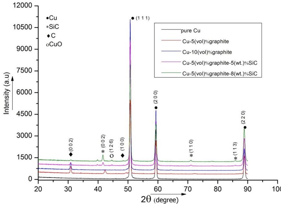
XRD spectra of fabricated composites
