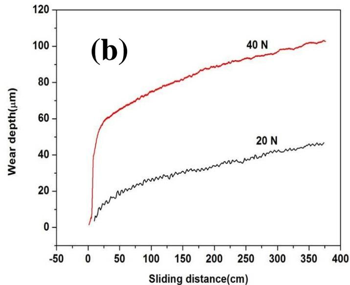
Variation of wear depth with sliding distance for (a) Cu-graphite, Cu-SiC and Cu-graphite-SiC composite (b) Cu-5 vol. % gr-5 wt. % SiC tested at 40 N and 20 N
