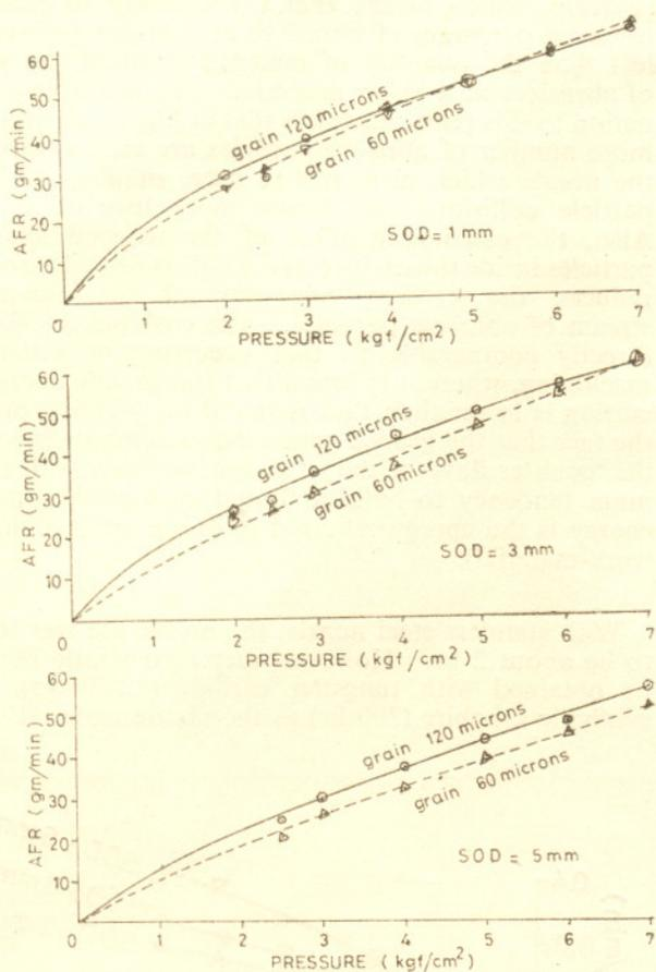
Fig 4 Variation of AFR with pressure: abrasive—SiC, nozzle dia—1.83 mm, work-material—porcelain
