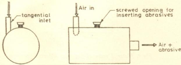
Fig 2 (c) Vortex type mixing chamber
