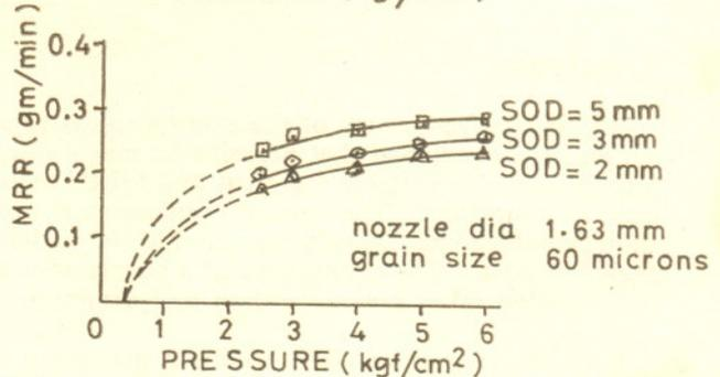
Fig 3 Variation of MRR with pressure abrasive—SiC, work material—porcelain
