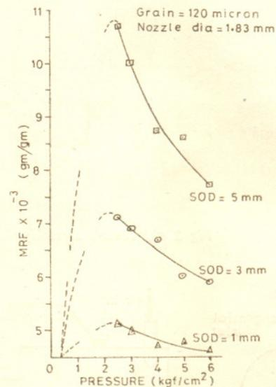
Fig 6 Material removal factor at different pressures
