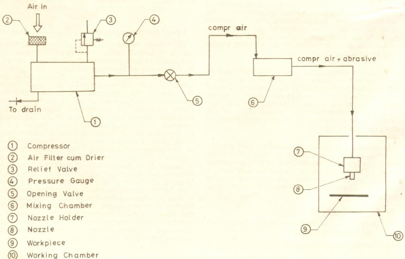
Fig 2 (a) Schematic diagram of experimental set-up
