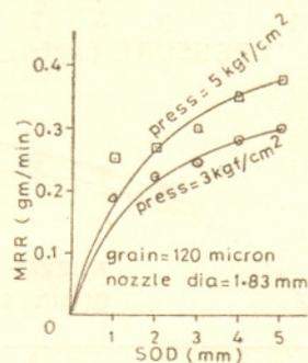
Fig 5 Variation of MRR with SOD
