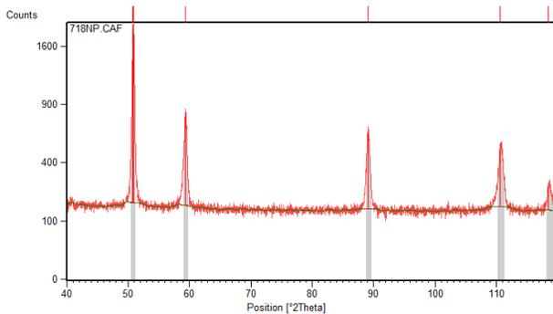
Figure 6. XRD spectra for ‘as received’ Inconel 718
