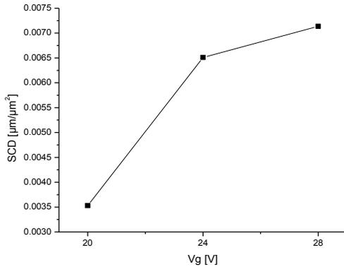
Figure 5. Effect of  $V_g$  on SCD for constant ( $I_p = 20A$ ) and ( $T_{on} = 300\mu s$ )
