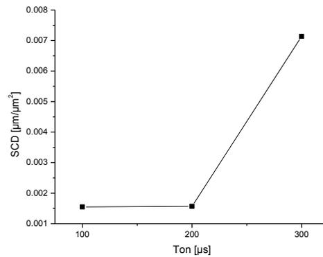
Figure 4. Effect of  $T_{on}$  on SCD for constant ( $I_p = 20A$ ) and ( $V_g = 28V$ )
