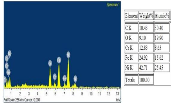
Figure 8. EDAX elemental spectra revealing chemical composition of ‘as received’ Inconel 718 parent material
