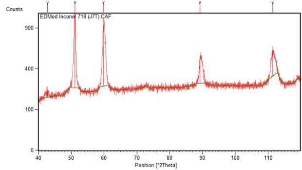
Figure 7. XRD spectra for EDMed work surface of Inconel 718 obtained at parameters setting [ $I_p=20A$ ,  $T_{on}=300\mu s$ ,  $V_g=24V$ ]
