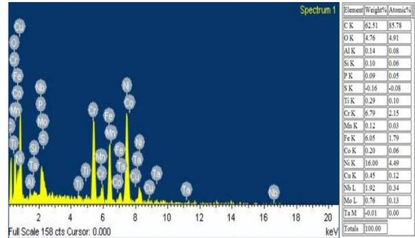
Figure 9. EDAX elemental spectra revealing chemical composition of the EDMed work surface of Inconel 718 obtained at parameters setting [ $I_p=20A$ ,  $T_{on}=300\mu s$ ,  $V_g=20V$ ]
