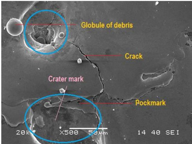
Figure 2. SEM image revealing irregularities on the surface of the EDMed Inconel 718 obtained at parameters setting [ $I_p=20A$ ;  $T_{on}=300\mu$ s;  $V_g=20V$ ]
