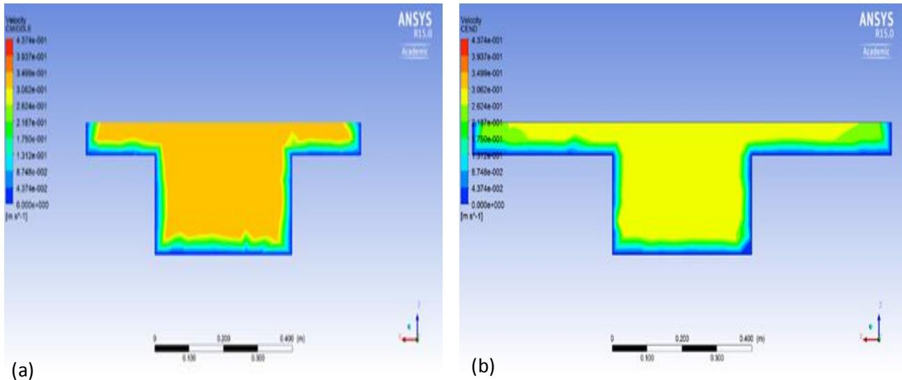
**Figure 4.** Contour of Computed (ANSYS-FLUENT) depth average velocity  $U_d$  in the rectangular non-prismatic diverging compound channel (a) middle and (b) end section for  $dr=.25$ .
