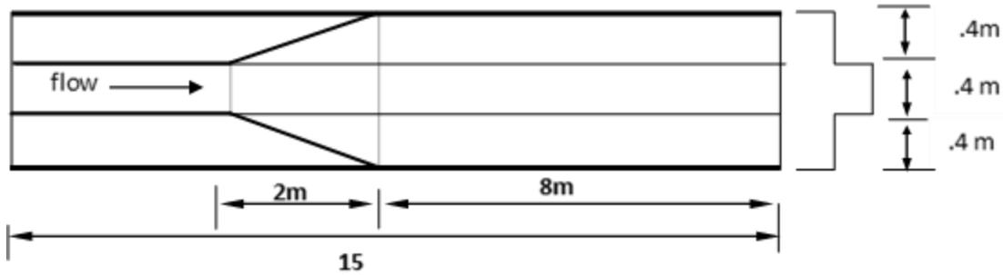
**Figure 1.** Schematic view of diverging channel ( $\Theta=11.31^\circ$ )
