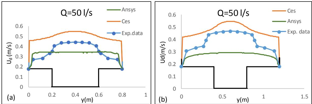
**Figure 3.** Comparison between computed (CES, ANSYS-FLUENT) and experimental depth average velocity  $U_d$  in the rectangular non-prismatic diverging compound channel (a) middle and (b) end section for  $dr=0.25$ .
