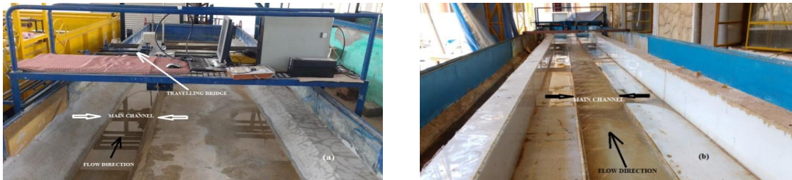
Figure 1. Photo of fabricated experimental channels, NITR (a) Trapezoidal (b) Rectangular
