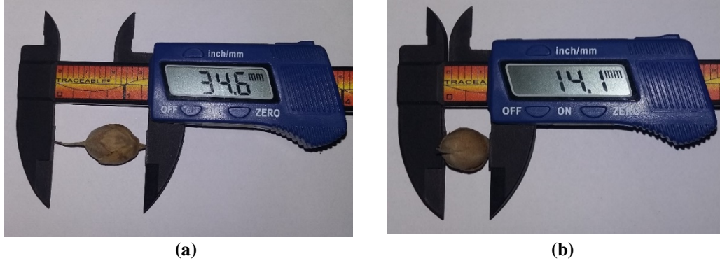
Figure.1 Representation of two major dimensions of sal seed; length (a), width (b).
