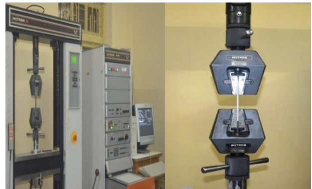
Fig. 1. UTM Instron 1195 and the loading arrangement
