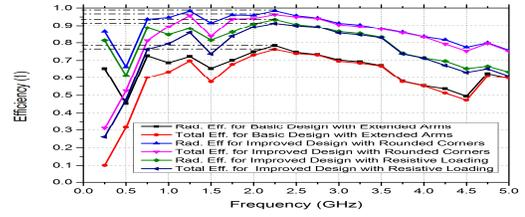
Fig. 10 Efficiency Vs frequency plots obtained from HFSS
