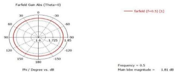
Fig. 12 H-Plane far field radiation pattern at  $f = 0.5$  GHz
