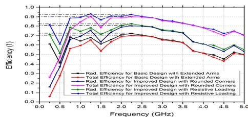
Fig. 9 Efficiency Vs frequency plots obtained from CST
