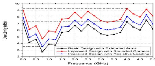
Fig. 8 Directivity Vs frequency plots obtained from HFSS
