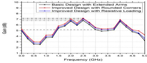
Fig. 6 Gain Vs frequency plots obtained from HFSS.
