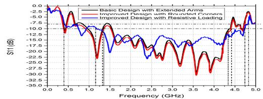
Fig. 4 Reflection coefficients Vs frequency plots obtained from HFSS.
