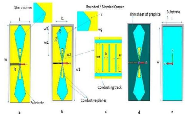
Fig. 2 Geometries of purposed antennas
