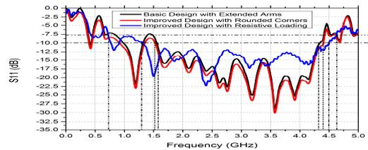
Fig. 3 Reflection coefficients Vs frequency plots obtained from CST.
