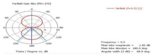
Fig. 11 E-Plane far field radiation pattern at  $f = 0.5$  GHz
