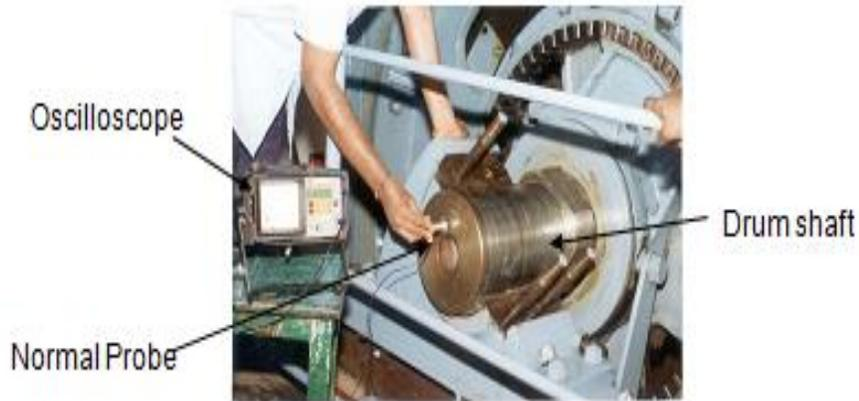
**Fig 4: Ultrasonic testing of typical drum shaft with normal probe**
