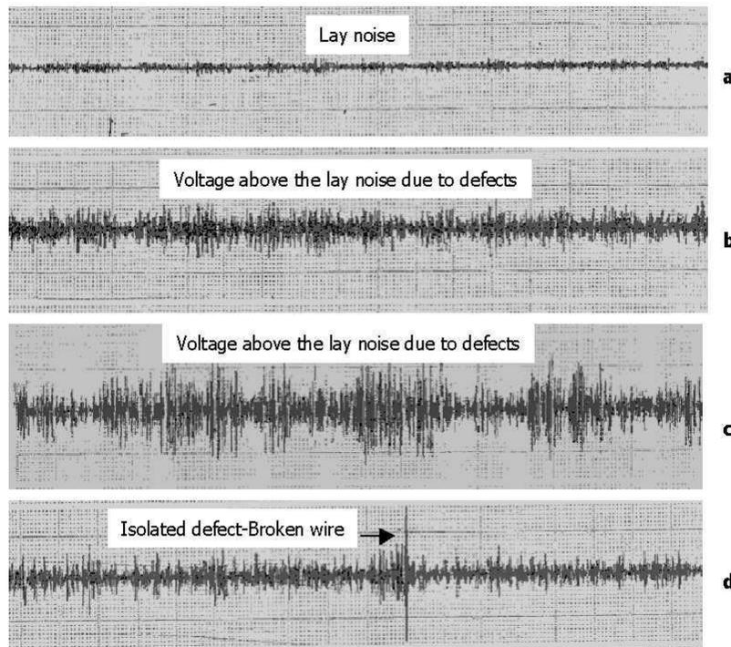
**Fig. 8: Defect pattern in a typical wire rope**
