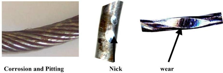
**Fig. 7: A typical rope sample with defects**
