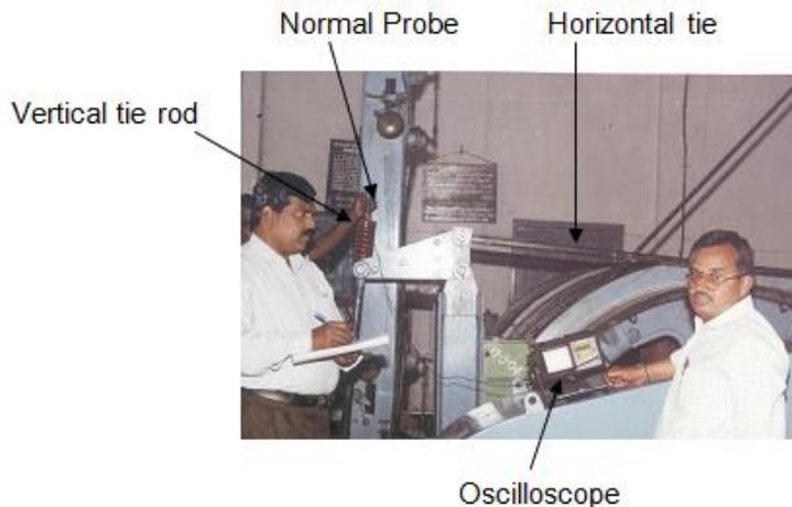
**Fig 5: Ultrasonic testing of typical vertical brake tie rod**
