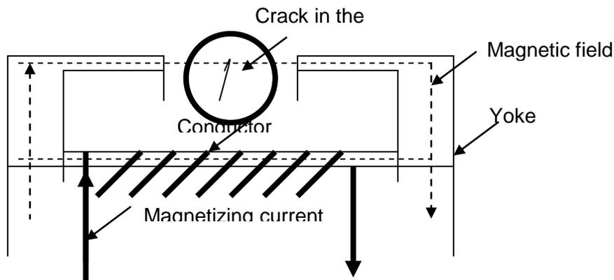
**Fig 2: Longitudinal Magnetization with yoke for magnetic particle testing**
