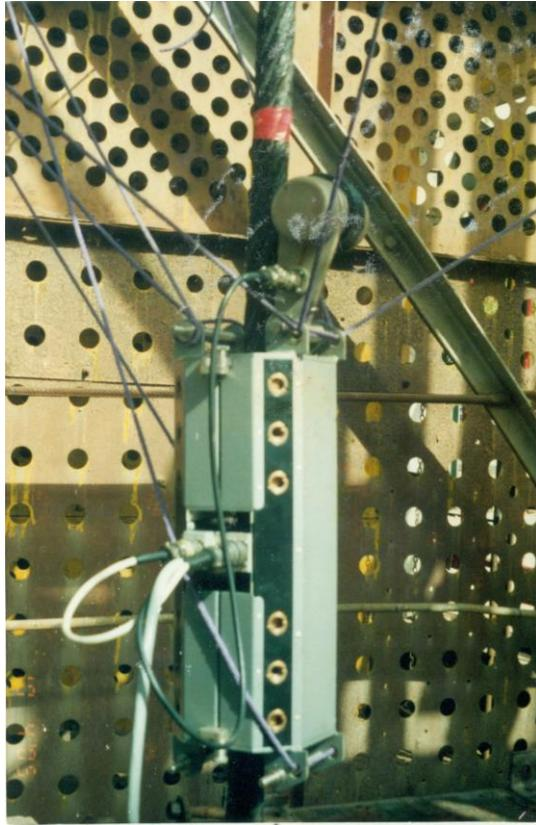
**Fig. 11: Rope defectograph commissioned in a typical underground mine for NDT test on winding rope**
