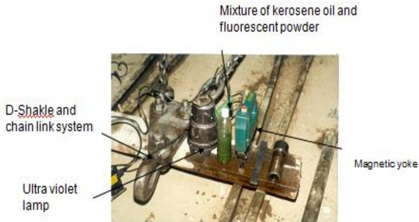
**Fig 3: Magnetic particle testing of components of suspension gear parts**
