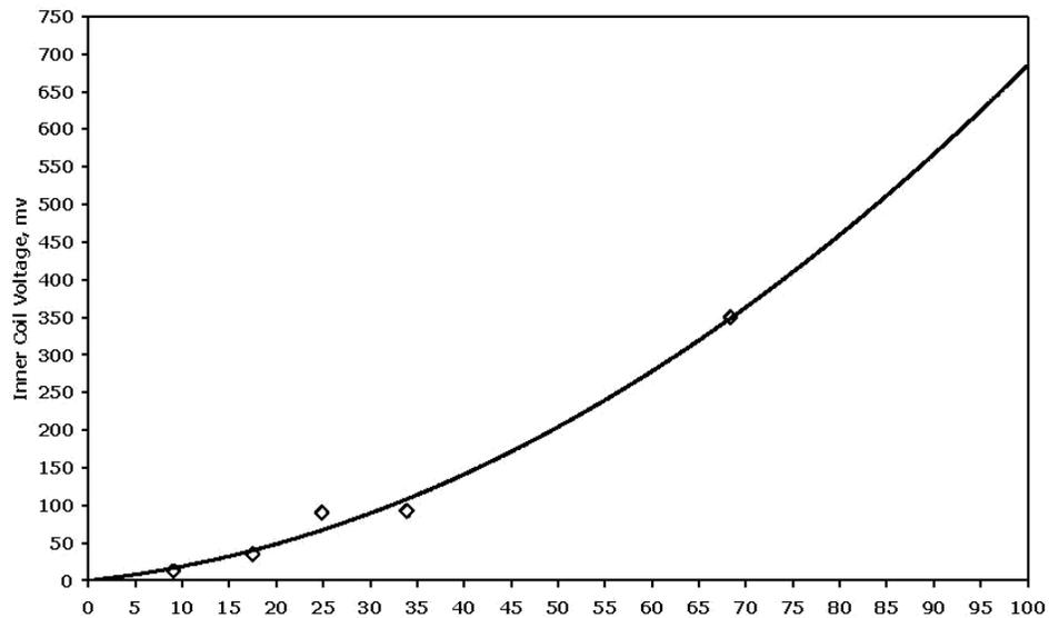
**Fig. 9: Calibration curve of wear Vs inner coil voltage**
