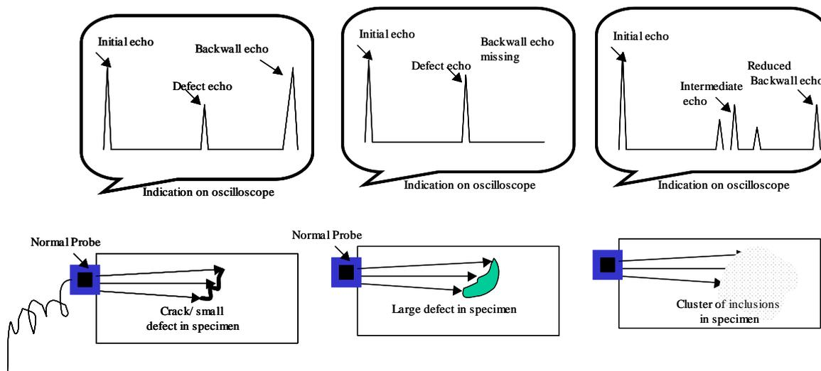
**Fig 1 : Principle of ultrasonic testing-Pulse echo method**
