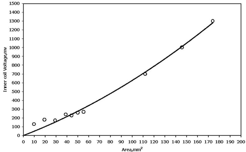
**Fig. 10: Calibration curve of area of broken wires Vs inner coil voltage**
