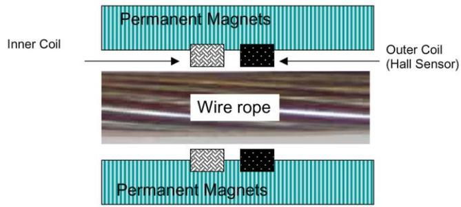
**Fig. 6: Schematic layout of equipment used in electromagnetic testing**
