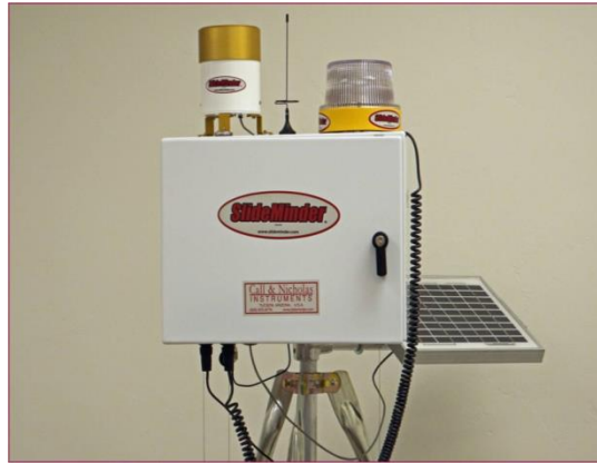
Fig.8. Slide Minder Wire line Extensometer System [9]
