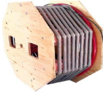
Fig.8. Shape Accel Array on shipping reel
