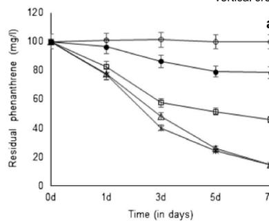
Fig. 6. Effect of biofilm growth phase on phenanthrene (a) and pyrene (b) degradation over the period of 7 days. Maximum degradation was observed when 48 h biofilm was used for degradation. Over the period of 7 days, degradation of both phenanthrene and pyrene was significantly affected by biofilm growth phase (two-way ANOVA  $P < 0.05$ ).
