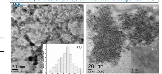
Fig. 9. Transmission electron micrographs of CdS NPs at different magnifications showing (a) CdS NPs embedded in EPS matrix, (b) exhibits the particle size in the range 20–40 nm in distribution histogram, (c) at higher magnification show large number of dispersed NPs and (d) lattice parameter of CdS NPs with high level of crystallinity at 5 nm resolution.
