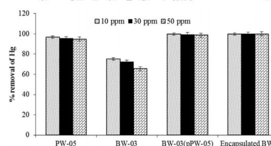
Fig. 7. In-vitro mercury removal potential of *B. thuringiensis* PW-05, *B. cereus* BW-03, transgenic *B. cereus* BW-03(pPW-05) and encapsulated *B. cereus* BW-03(pPW-05) with various concentrations of  $HgCl_2$ .
