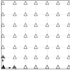
Fig. 4: Beacon node at the corner of grid
