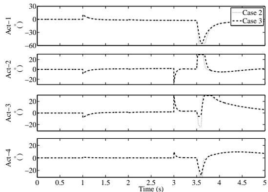
Fig. 3: Actuator responses of closed-loop ADMIRE system models.
