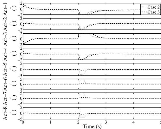
Fig. 5: Actuator response of closed-loop SLV system.
