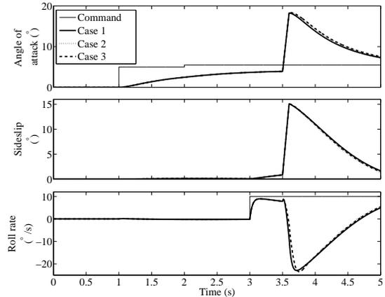
Fig. 2: Output response of closed-loop ADMIRE system models.
