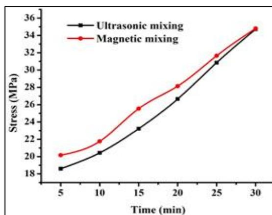
Fig. 1: Effect of Mixing Variations on Tensile Strength.
