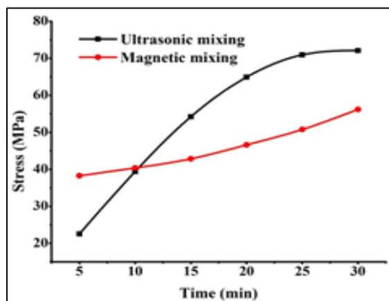
**Fig. 3:** Effect of Mixing Variations on Flexural Strength.
