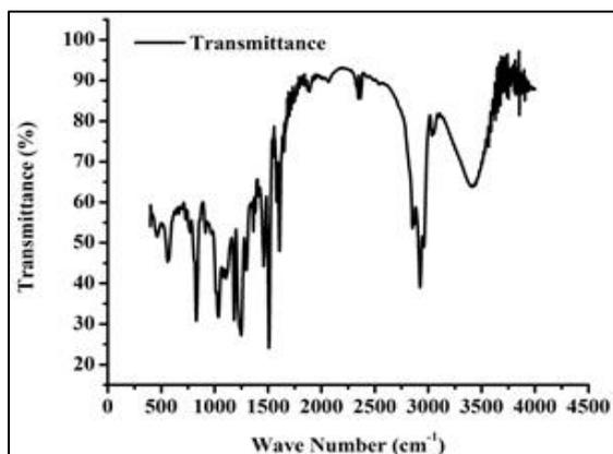
Fig. 7: IR Spectra of the 10% Fly Ash And 90% Epoxy Resin.
