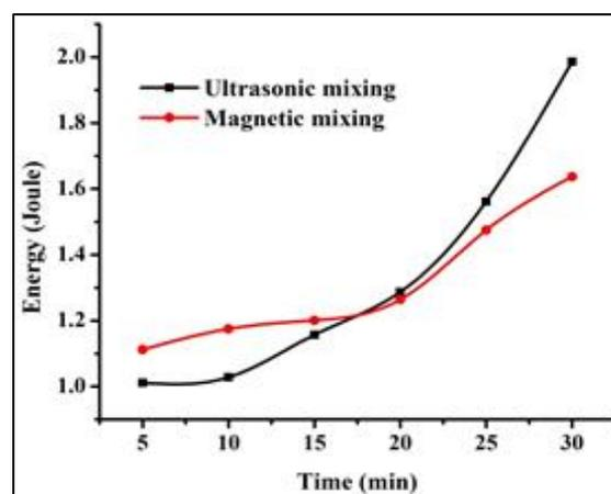
Fig. 5: Effect of Mixing Variations on Impact Strength.
