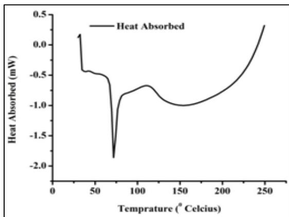
Fig. 8: DSC Thermograph of 10% Fly Ash and 90% Epoxy Resin Mix.
