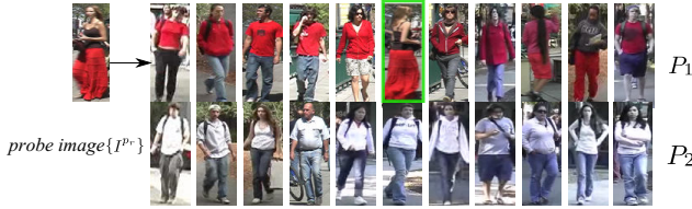
Fig. 4: Example of prototype formation on few images of gallery set of VIPeR Dataset. P_1 and P_2 denote the prototypes. P_1 and P_2 represent the images with similar appearances. Based on the feature of the probe image, it only compares with the images belonging to prototype P_1 . The green bounding box signifies as true match.
