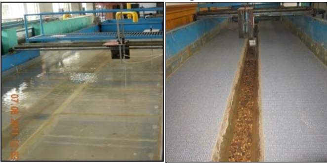
Figure 1. Details of straight smooth and rough channel
