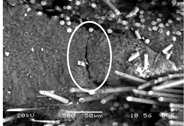
Fig 6: Scanning electron micrograph at ambient 1 mm/min and 800 mm/min shows steps and welts as well as matrix cracking respectively.
