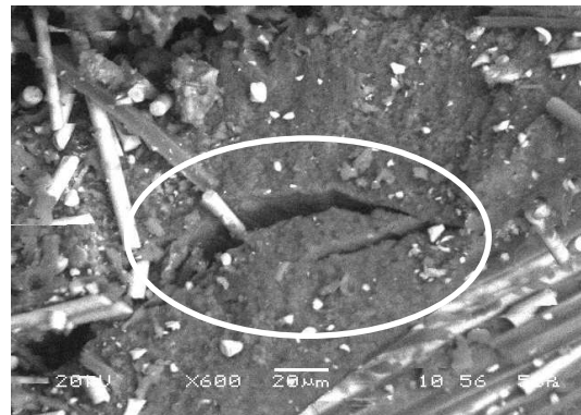
Fig 7: Thermal conditioning sample at 1 mm/min and 800 mm/min showing fibre/matrix debonding and macromatrix cracking.
