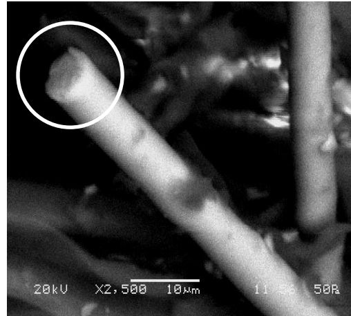
Fig 4: Matrix micro cracking and brittle fracture of fiber at -50°C temperature at 1 mm/min and 800 mm/min.
