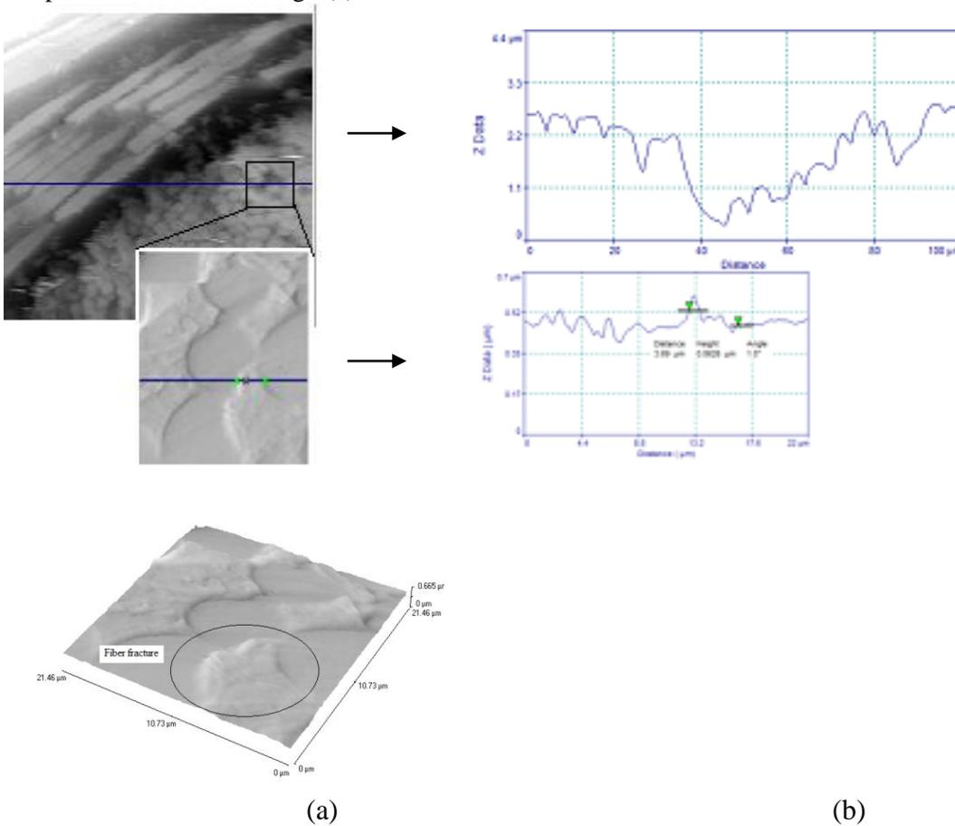
Fig 1: AFM topography images of untreated GFRP composites (a) line analysis of image (b) 3D image analysis
