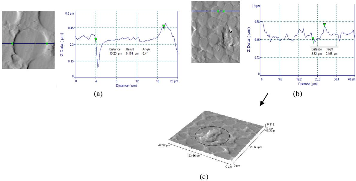
Fig 4: AFM topography image of treated GFRP adhesion failure after thermal conditioning treatment.
