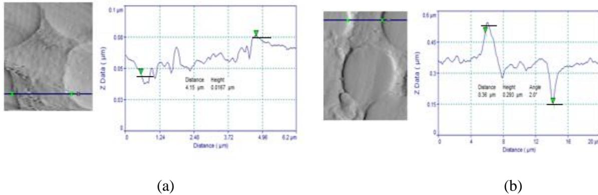
Fig 2: AFM topography image of treated GFRP interphase failure after treatment.
