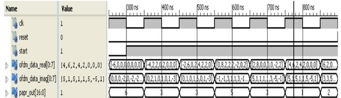
Fig. 6. Test-bench waveform for PAPR calculation.
