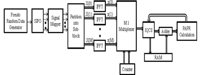
Fig. 4. VHDL implementation of the modified partial transmit sequence technique (CS-PTS).
