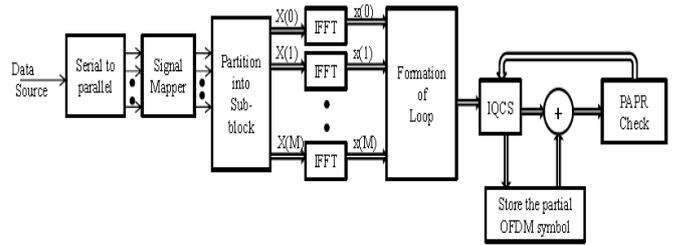
Fig. 2. PAPR reduction by modified partial transmit sequence technique (CS-PTS).
