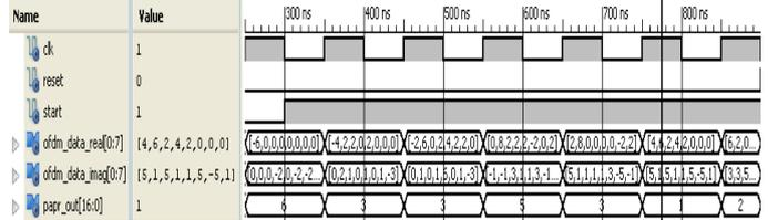
Fig. 6. Test-bench waveform for PAPR calculation.
