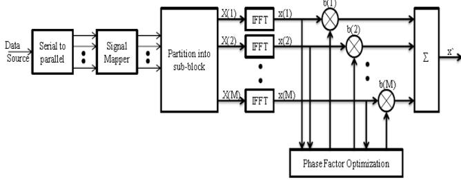
Fig. 1. PAPR reduction by conventional partial transmit sequence technique (C-PTS).
