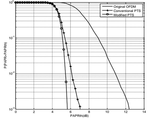
Fig. 3. CCDF of PAPR with N=64, M=4 and P=8, Q=8 for OFDM without PTS, with conventional PTS and with modified PTS.
