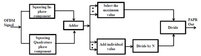
Fig. 5. Block Diagram for PAPR calculation in VHDL.
