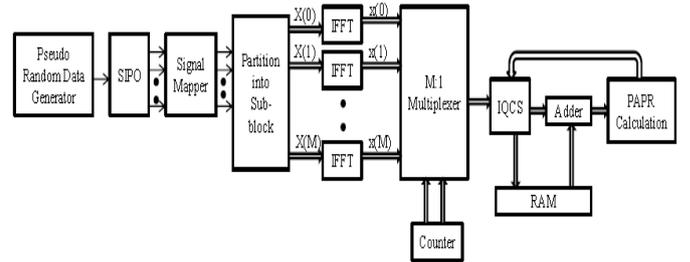
Fig. 4. VHDL implementation of the modified partial transmit sequence technique (CS-PTS).
